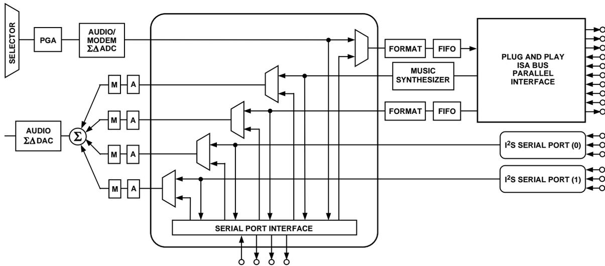
Figure 14. DSP Serial Port
