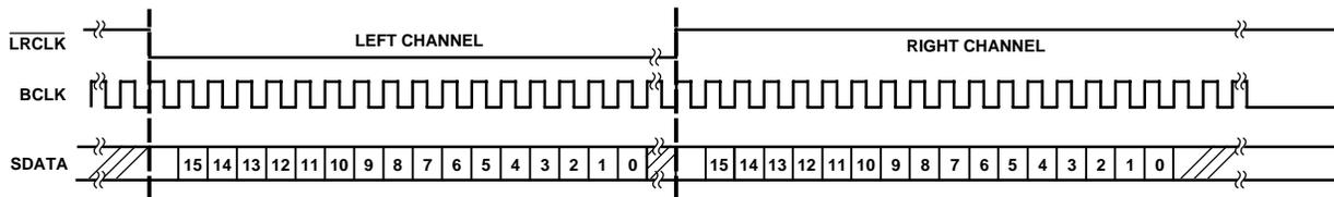
Figure 10. Serial Interface I<sup>2</sup>S-Justified Mode
