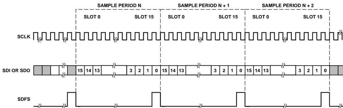
Figure 12. DSP Serial Interface (Default Frame Rate)
