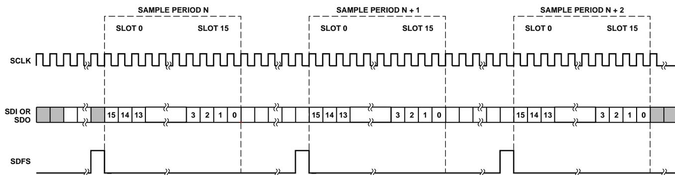
Figure 13. DSP Serial Interface (User Programmed Frame Rate)
