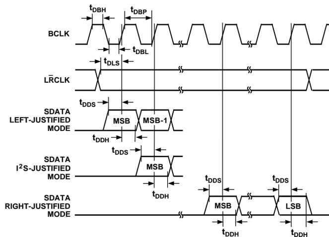
Figure 7. I²S Serial Port Timing
