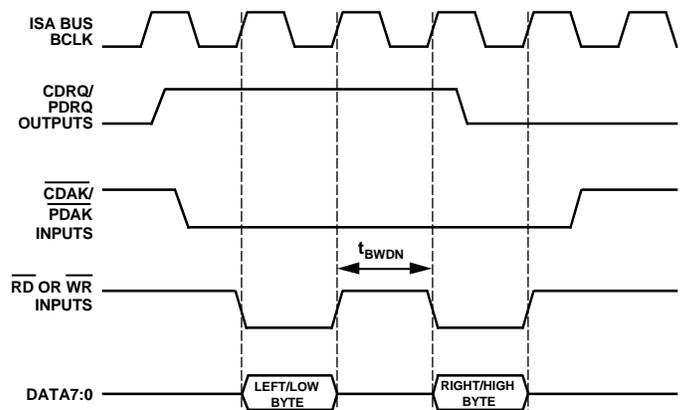
Figure 15. 8-Bit Stereo or 16-Bit Mono DMA Cycle
