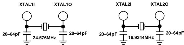
Figure 23. Crystal Connections
