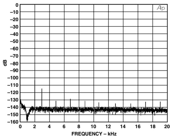
Figure 12. 1 kHz Tone at  $-0.5$  dBFS (8K-Point FFT)
