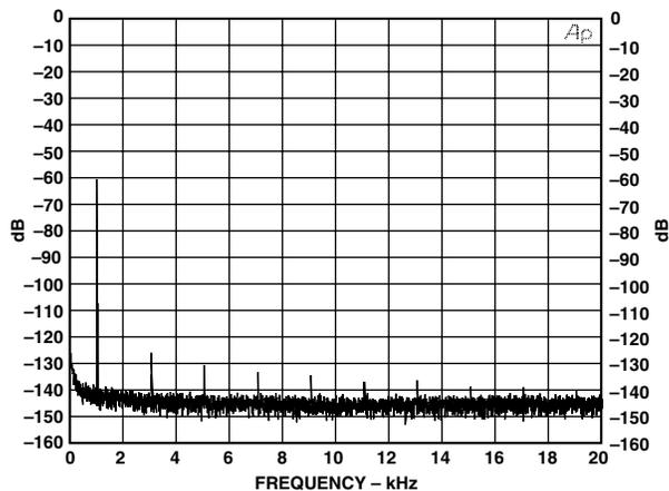
Figure 14. Dynamic Range: 1 kHz at  $-60$  dB
