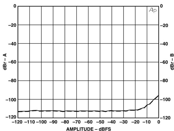
Figure 15. THD+N vs. Amplitude at 1 kHz
