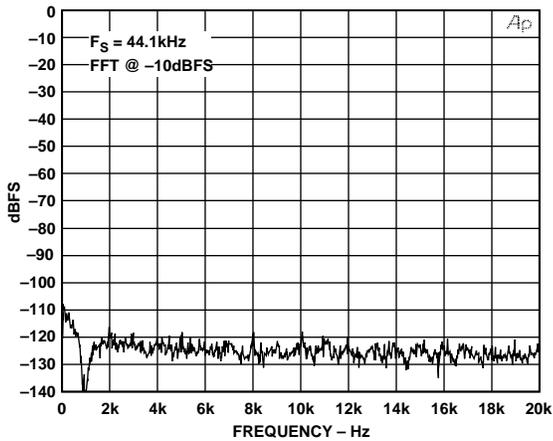
Figure 25. 1 kHz Tone at -10 dBFS (16K-Point FFT)
