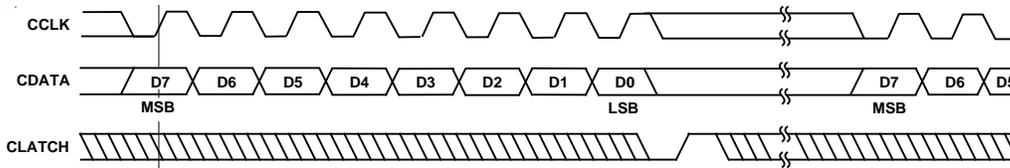
Figure 7. Serial Control Port Timing
