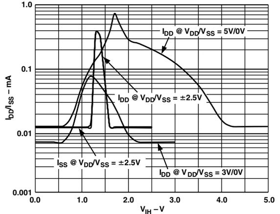
TPC 5. Supply Current vs. Logic Input Voltage
