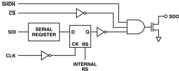
Figure 4. Detail SDO Output Schematic of the AD5207
