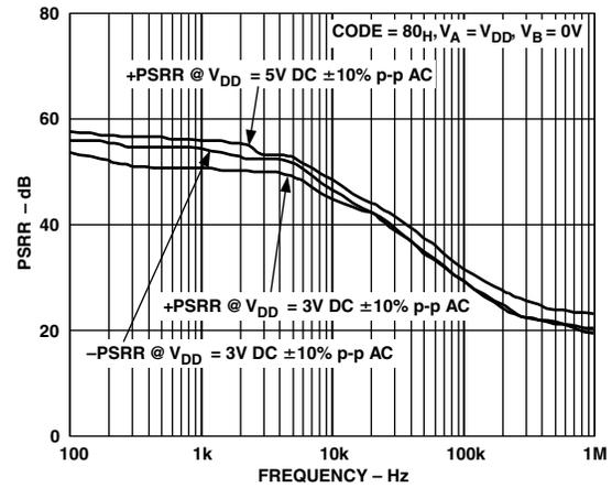
TPC 11. Power Supply Rejection Ratio vs. Frequency
