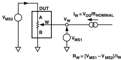
Figure 12. Wiper Resistance Test Circuit
