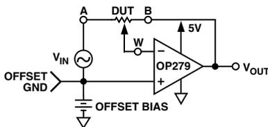
Figure 14. Inverting Gain Test Circuit
