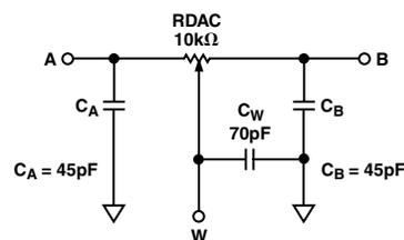
Figure 9. RDAC Circuit Simulation Model for RDAC = 10 kΩ
