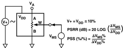
Figure 13. Power Supply Sensitivity Test Circuit (PSS, PSSR)
