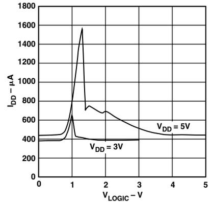
Figure 19. Supply Current vs. Logic Input Voltage
