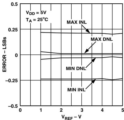
Figure 11. AD5334 INL and DNL Error vs.  $V_{REF}$
