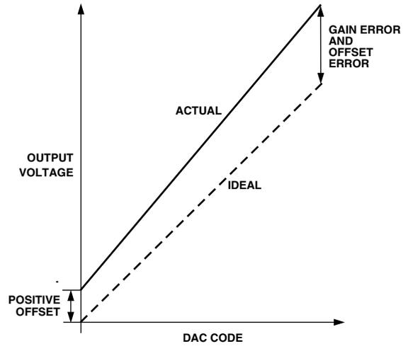
Figure 3. Positive Offset Error and Gain Error
