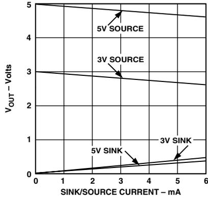
Figure 15.  $V_{OUT}$  Source and Sink Current Capability
