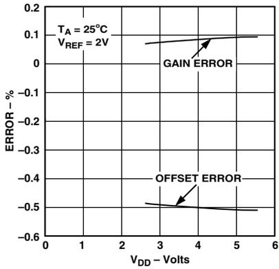
Figure 14. Offset Error and Gain Error vs.  $V_{DD}$
