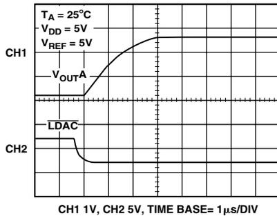
Figure 20. Half-Scale Settling (1/4 to 3/4 Scale Code Change)
