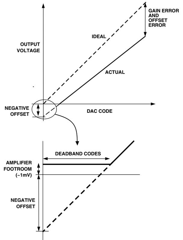
Figure 4. Negative Offset Error and Gain Error
