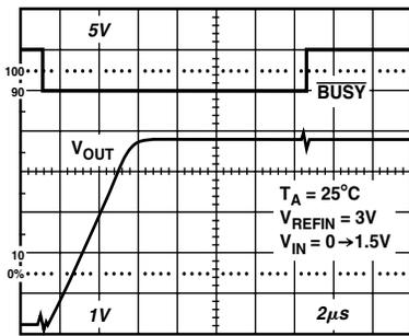
Figure 9. Acquisition Time and Output Settling Time
