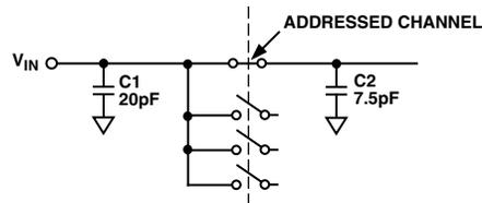
Figure 11. Analog Input Circuit
