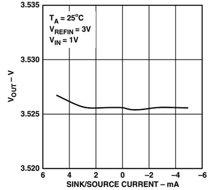
Figure 8.  $V_{OUT}$  Source and Sink Capability
