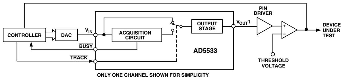
Figure 12. Typical ATE Circuit Using  $\overline{TRACK}$  Input
