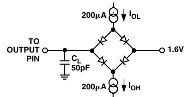
Figure 2. Load Circuit for D<sub>OUT</sub> Timing Specifications
