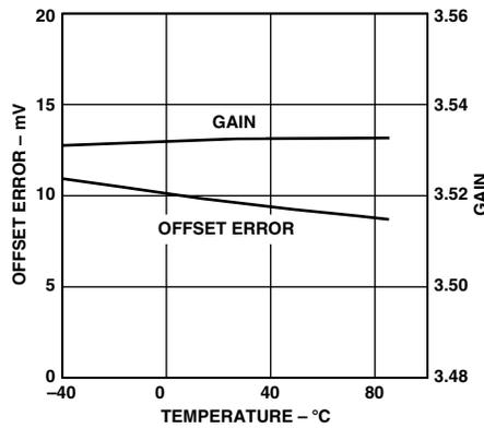
Figure 7. Offset Error and Gain vs. Temperature
