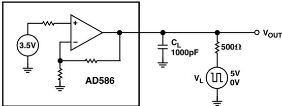
Figure 7a. Capacitive Load Transient Response Test Circuit
