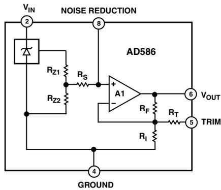
NOTE: PINS 1, 3, AND 7 ARE INTERNAL TEST POINTS. MAKE NO CONNECTIONS TO THESE POINTS.
