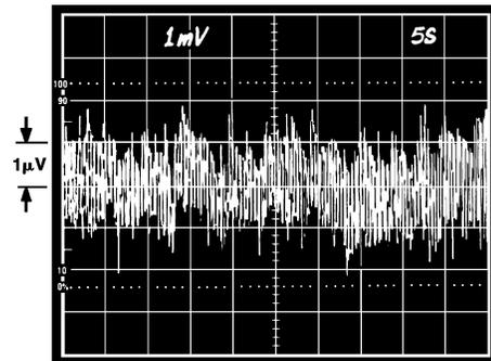
Figure 3. 0.1 Hz to 10 Hz Noise
