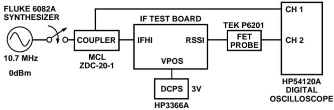
Figure 12. Test Circuit for RSSI Pulse Response/RSSI Rise Time (Figure 11)
