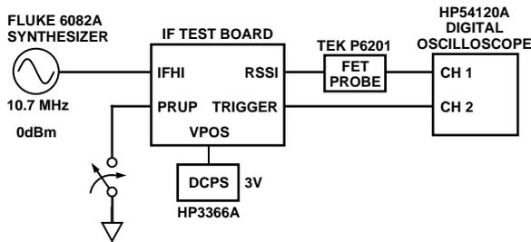
Figure 10. Test Circuit for RSSI Power-Up Response (Figure 9)
