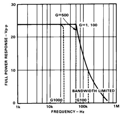
Figure 5. Large Signal Frequency Response
