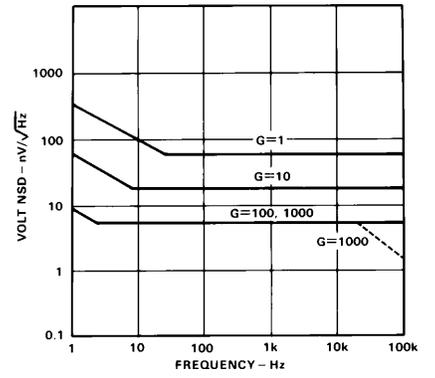
Figure 14. RTI Noise Spectral Density vs. Gain
