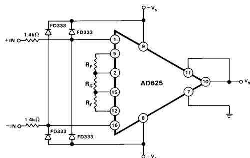
Figure 26a. Input Protection Circuit
