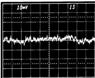
Figure 18. Low Frequency Voltage Noise,  $G = 1000$  (System Gain = 100,000)
