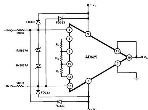
Figure 26b. Input Protection Circuit for  $G > 5$
