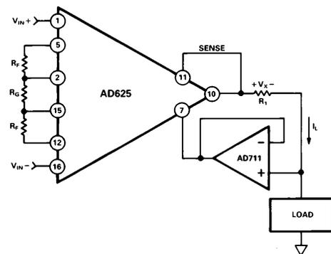
Figure 31. Voltage-to-Current Converter
