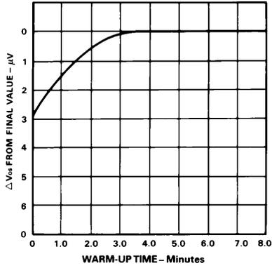
Figure 7. Offset Voltage, RTI, Turn On Drift
