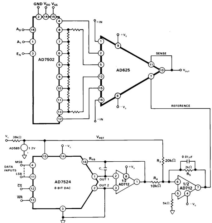
Figure 30. Software Controllable Offset
