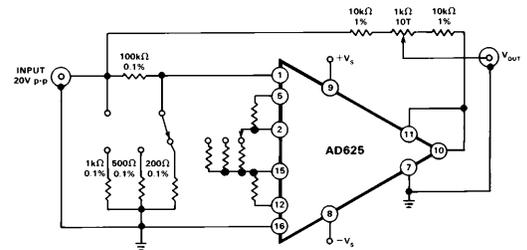
Figure 23. Settling Time Test Circuit
