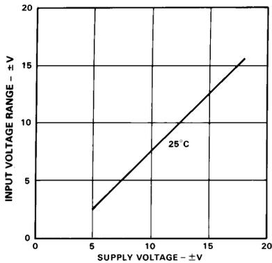
Figure 1. Input Voltage Range vs. Supply Voltage,  $G = 1$
