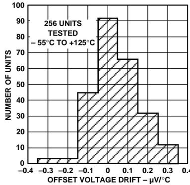
Figure 5. Typical Distribution of Offset Voltage Drift
