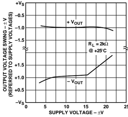
Figure 2. Output Voltage Swing vs. Supply Voltage
