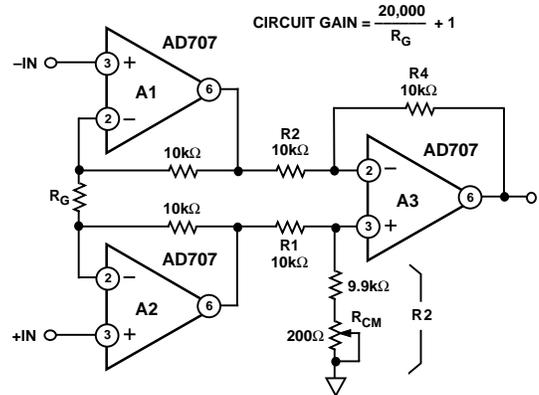
Figure 24. A 3 Op Amp Instrumentation Amplifier
