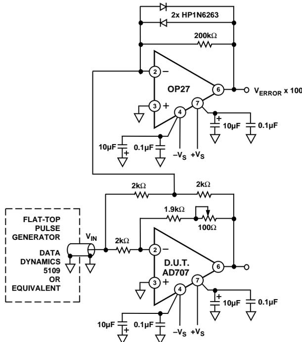
Figure 23. Op Amp Settling Time Test Circuit
