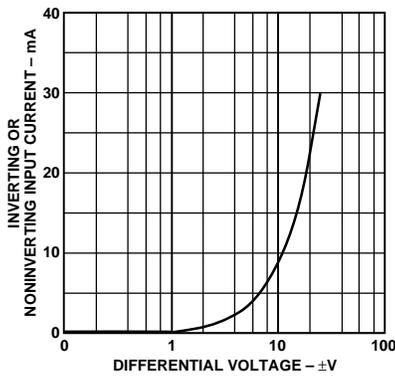
Figure 7. Input Current vs. Differential Input Voltage
