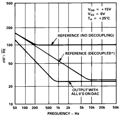
\*REFERENCE DECOUPLING COMPONENTS AS PER FIGURE 8
