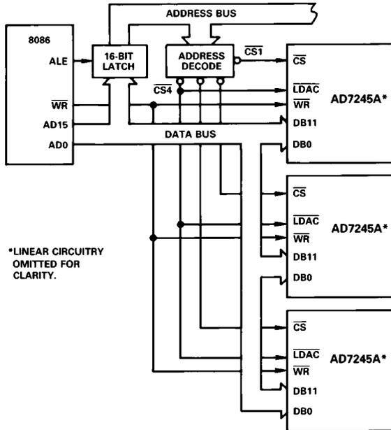
Figure 13. AD7245A to 8086 Multiple DAC Interface
