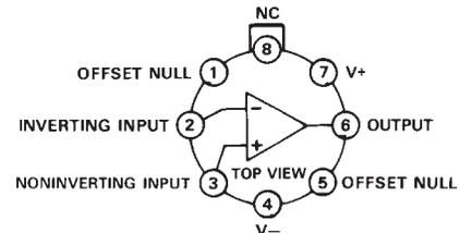
NOTE: PIN 4 CONNECTED TO CASE
