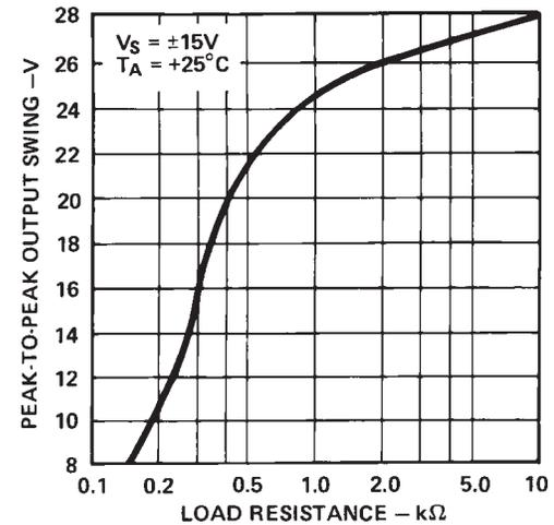
Figure 11. Output Voltage Swing vs. Load Resistance
