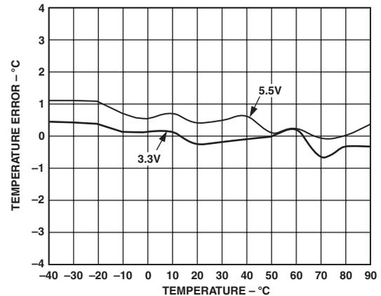
Figure 14. Typical Temperature Error @ 3.3 V and 5.5 V
