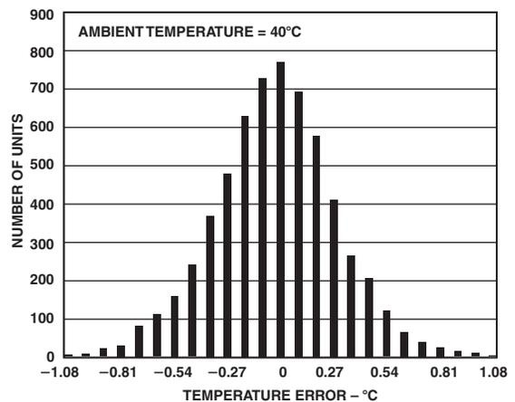
Figure 15. Ambient Temperature Error @ 3 V
