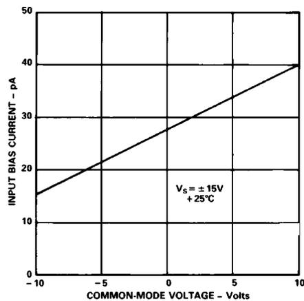
Figure 7. Input Bias Current vs. Common-Mode Voltage
