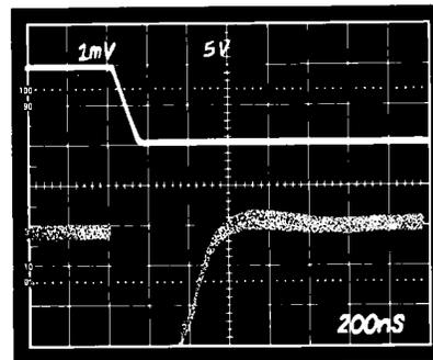
Figure 27. Settling Characteristics 0 to -10 V Step
