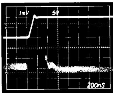
Figure 26. Settling Characteristics 0 to +10 V Step
