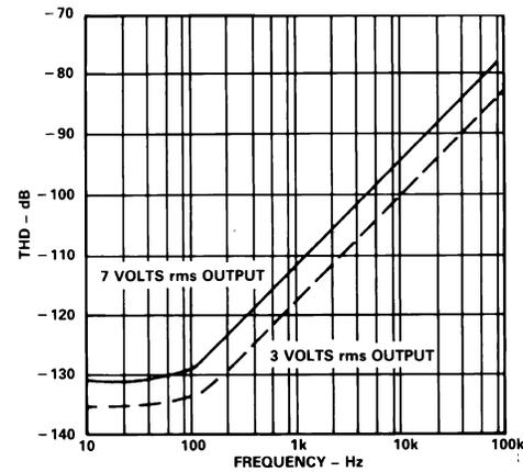
Figure 16. Total Harmonic Distortion vs. Frequency, Circuit of Figure 20
