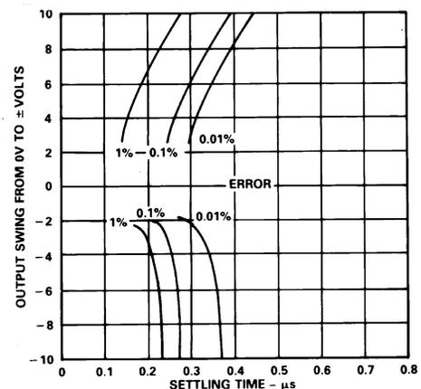
Figure 15. Output Swing and Error vs. Settling Time
