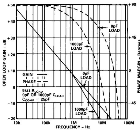
Figure 11. Open Loop Gain and Phase Margin vs. Frequency
