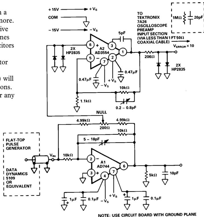
Figure 25. Settling Time Test Circuit
