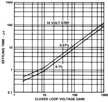
Figure 19. Settling Time vs. Closed Loop Voltage Gain
