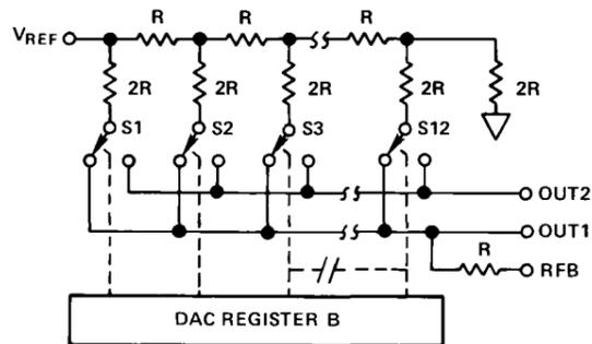
Figure 1. AD7543 Functional Diagram
