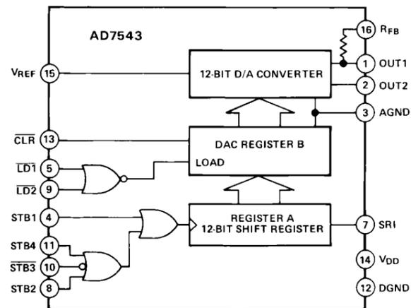
Initialization is simplified by the use of the CLR input which provides an asynchronous reset of Register B.
