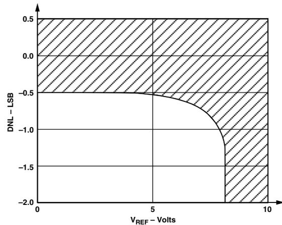
Figure 9. Differential Nonlinearity vs. Reference Voltage for Figure 7 Circuit.  $V_{DD} = 15$  Volts. Shaded Area Shows Range of Values of Differential Nonlinearity that Typically Occur for L, C and U Grades.
