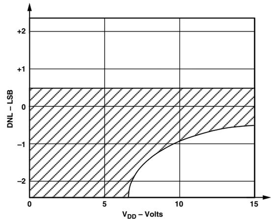
Figure 8. Differential Nonlinearity vs.  $V_{DD}$  for Figure 7 Circuit. Reference Voltage = 2.5 Volts. Shaded Area Shows Range of Values of Differential Nonlinearity that Typically Occur for L, C and U Grades.
