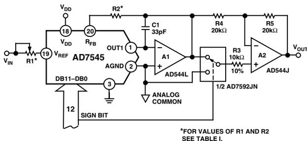
Figure 6. 12-Bit Plus Sign Magnitude D/A Converter
