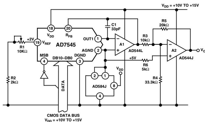
Figure 10. Single Supply "Bipolar" Twos Complement D/A Converter
