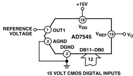
Figure 7. Single Supply Operation Using Voltage Switching Mode
