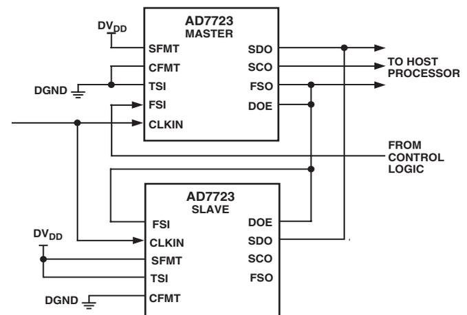
Figure 24. Serial Mode 1 Connection for Two-Channel Multiplexed Operation
