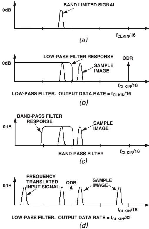
Figure 10. Band-Pass Operation
