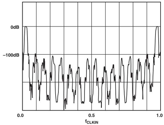
Figure 11c. Band-Pass Filter Decimate by 32
