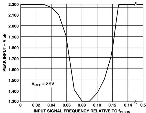
Figure 14. Peak Input Signal Level vs. Signal Frequency
