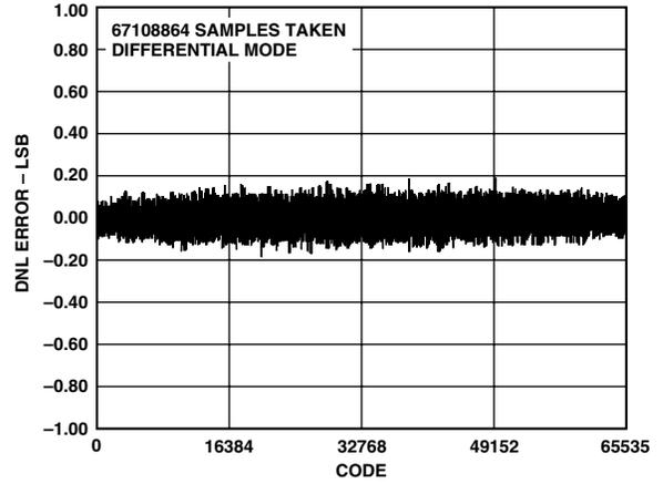
TPC 10. Differential Nonlinearity (Output Data Rate = 600 kHz)
