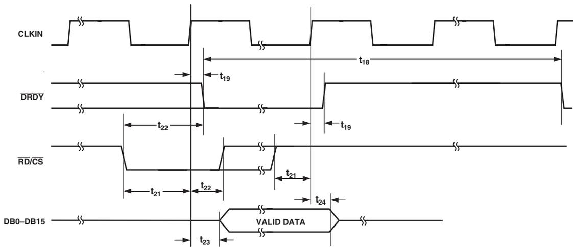
Figure 7b. Parallel Mode Read Timing,  $\overline{CS} = \overline{RD}$
