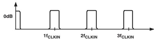
Figure 12a. Digital Filter Frequency Response
