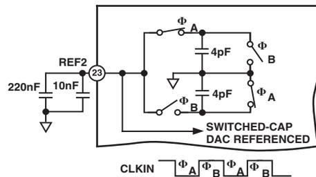
Figure 20. REF2 Equivalent Input Circuit
