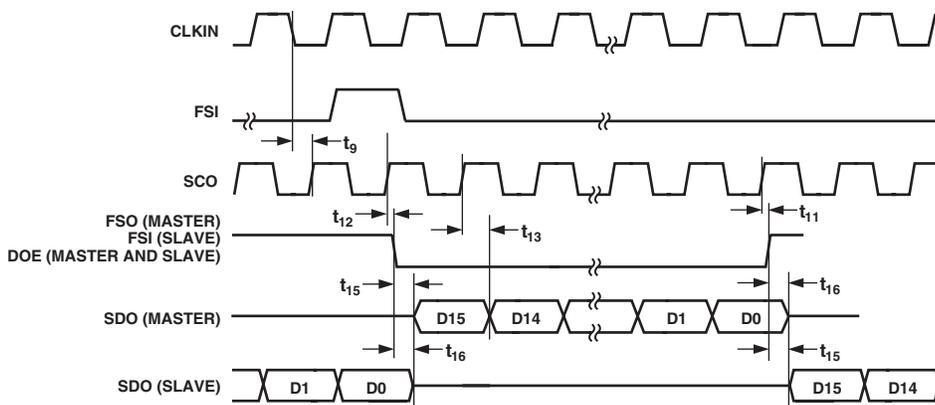
Figure 25. Serial Mode 1 Timing for Two-Channel Multiplexed Operation
