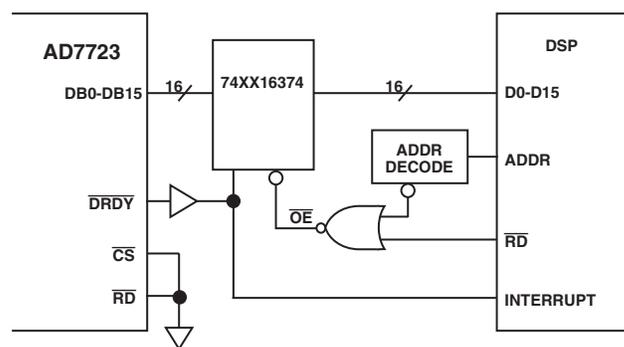
Figure 23. Parallel Interface Connection
