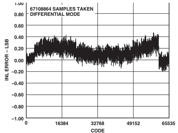
TPC 12. Integral Nonlinearity (Output Data Rate = 600 kHz)
