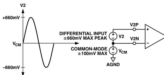
Figure 23. Maximum Signal Levels, Channel 2
