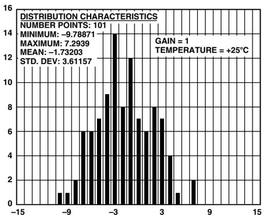
Figure 14. Channel 1 Offset Distribution (Gain = 1)
