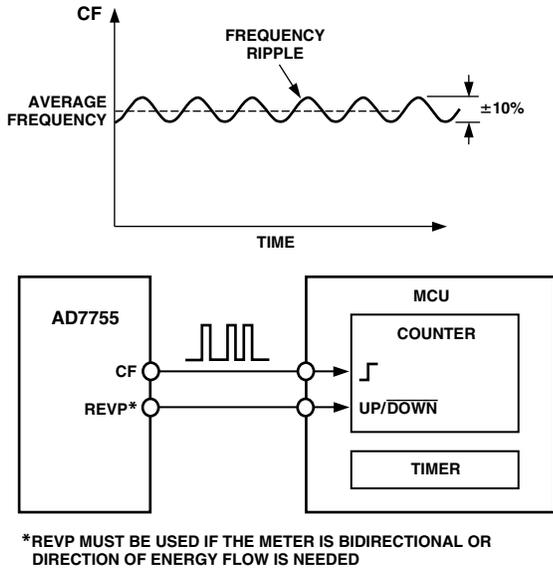
Figure 31. Interfacing the AD7755 to an MCU
