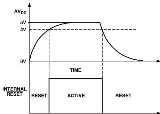
Figure 26. On-Chip Power Supply Monitor
