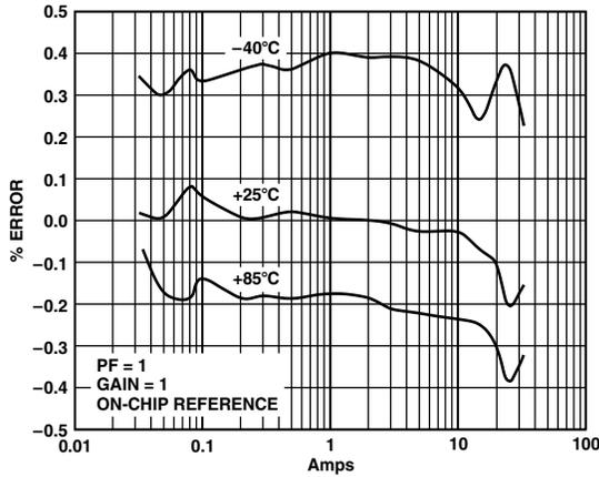
Figure 2. Error as a % of Reading (Gain = 1)
