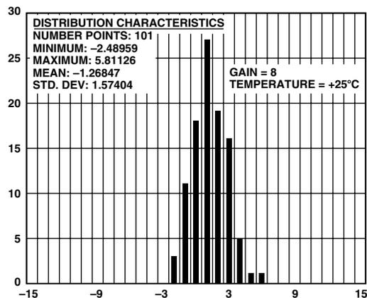
Figure 17. Channel 1 Offset Distribution (Gain = 8)
