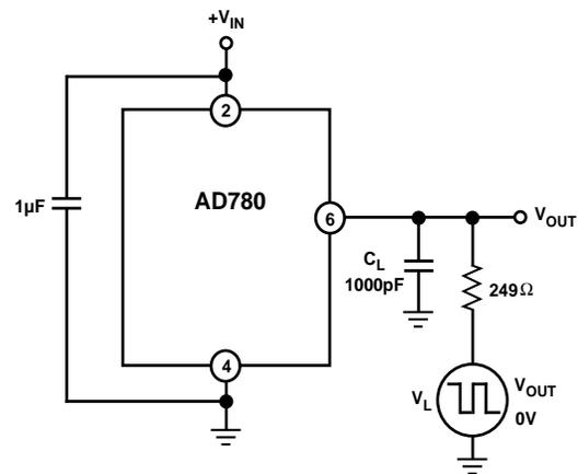
Figure 13a. Capacitive Load Transient Response Test Circuit
