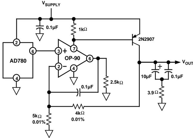
Figure 17. +4.5 V Reference from a Single +5 V Supply
