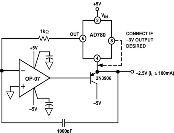
Figure 19. -2.5 V High Load Current Reference
