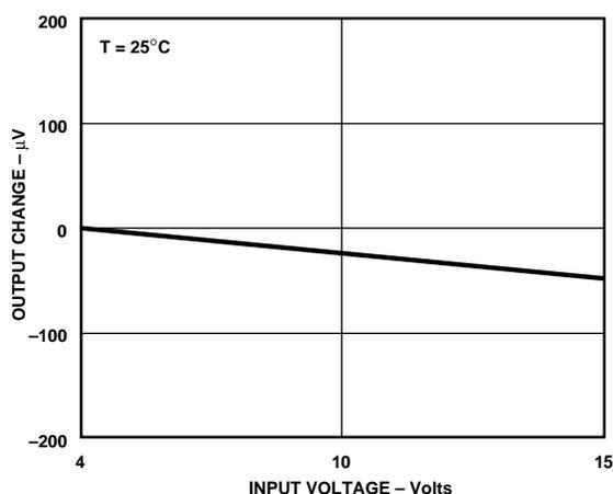
Figure 14. Output Voltage Change vs. Input Voltage
