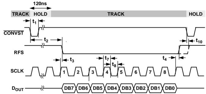
Figure 4. Track-and-Hold Timing
