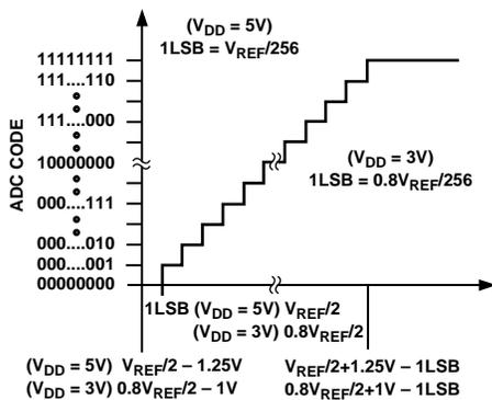
Figure 6. Transfer Characteristic
