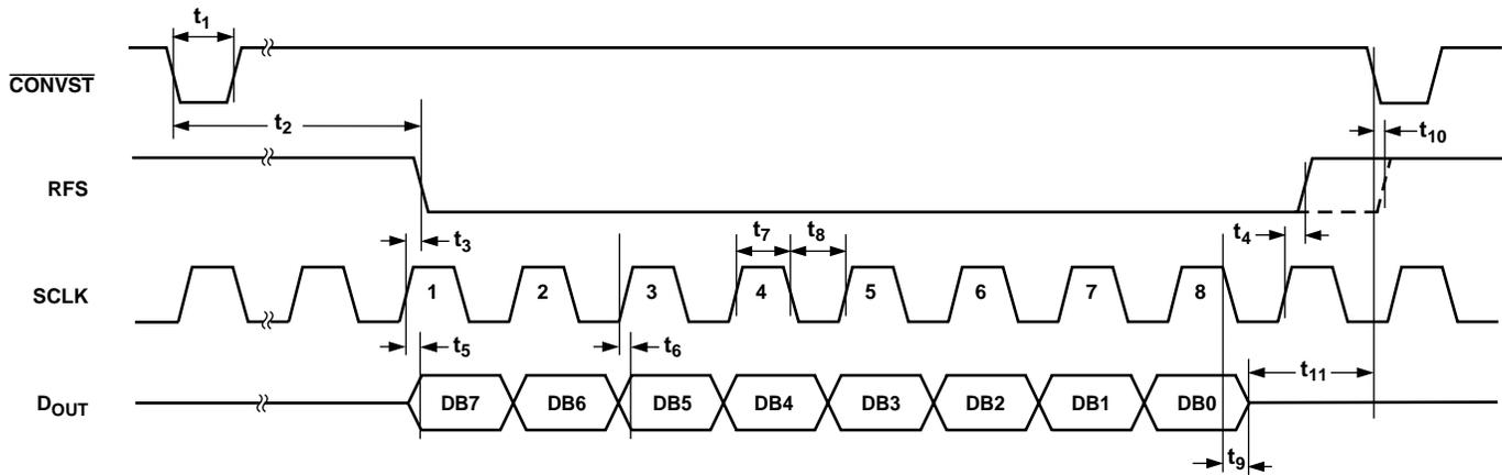
Figure 15. Serial Timing
