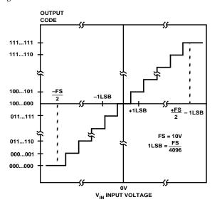
Figure 7. Bipolar Transfer Characteristic
