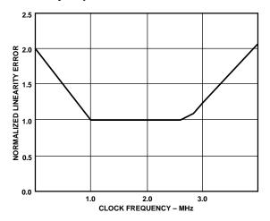
Figure 8. Normalized Linearity Error vs. Clock Frequency
