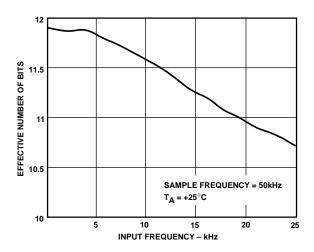
Figure 11. Effective Number of Bits vs. Frequency
