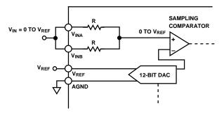
Figure 4. 0 to V<sub>REF</sub> Unipolar Input Configuration
