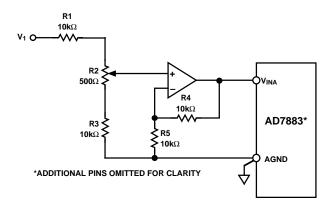
Figure 9. Offset and Full-Scale Adjust Circuit
