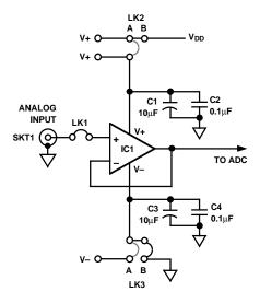
Figure 13. Analog Input Buffering
