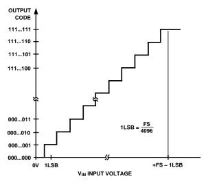
Figure 6. Unipolar Transfer Characteristics
