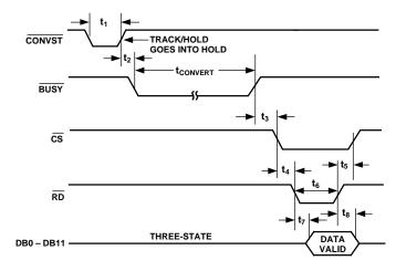
Figure 1. Timing Diagram
