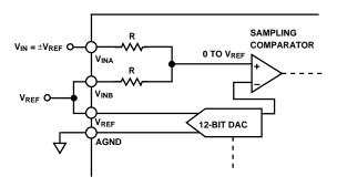
Figure 5.  $\pm V_{REF}$  Bipolar Input Configuration
