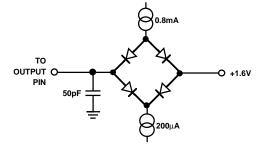
Figure 2. Load Circuit for Access and Relinquish Time
