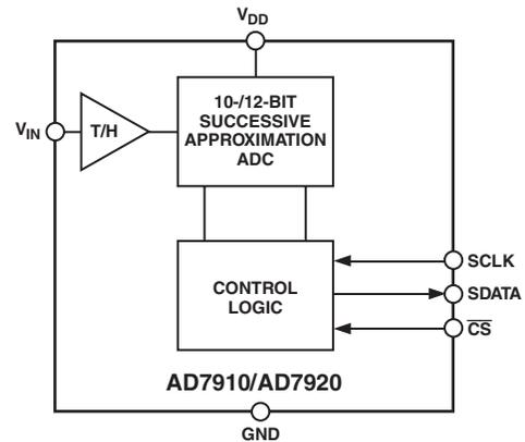
The reference for the part is taken internally from  $V_{DD}$ . This allows the widest dynamic input range to the ADC. Thus the analog input range for the part is 0 to  $V_{DD}$ . The conversion rate is determined by the SCLK.
