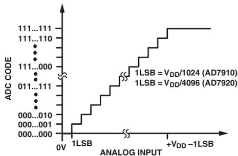
Figure 6. Transfer Characteristic
