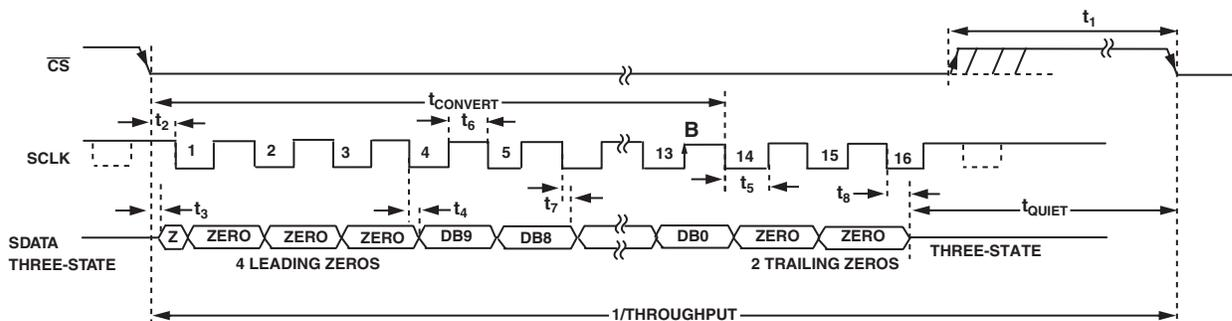
Figure 14. AD7910 Serial Interface Timing Diagram
