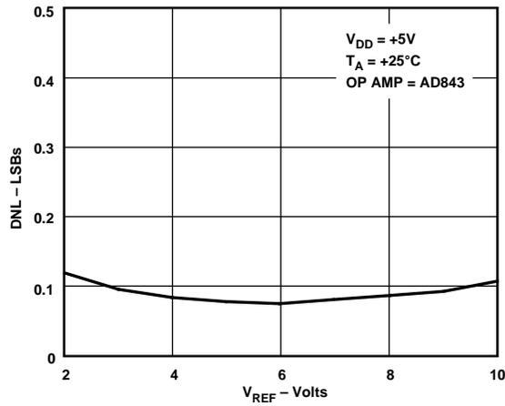
Figure 5. Differential Nonlinearity Error vs.  $V_{REF}$  (Normal Mode)
