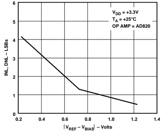
Figure 8. Linearity Error vs.  $V_{REF}$  (Biased Mode)
