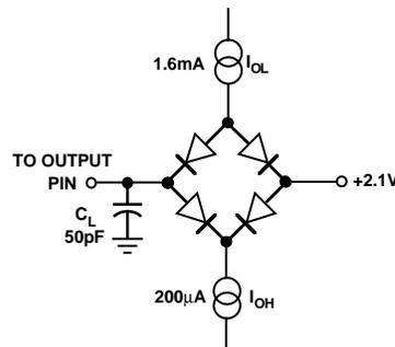
Figure 2. Load Circuit for Digital Output Timing Specifications
