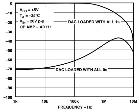
Figure 12. Multiplying Frequency Response vs. Digital Code
