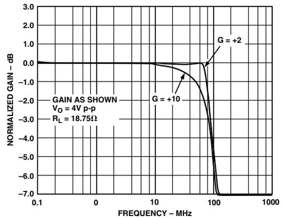
Figure 20. Large Signal Frequency Response;  $V_O = 4 V p-p$
