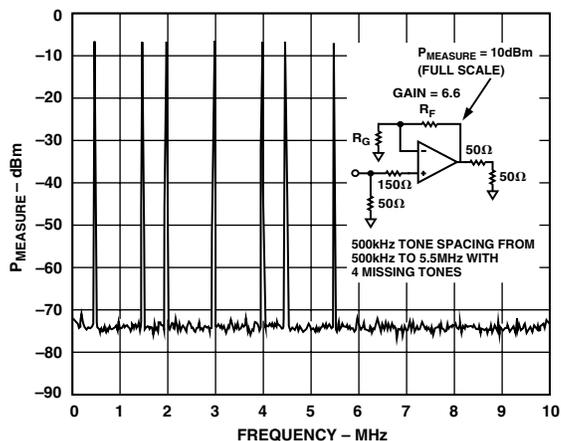
Figure 12. Multitone Distortion;  $R_L = 100 \Omega$
