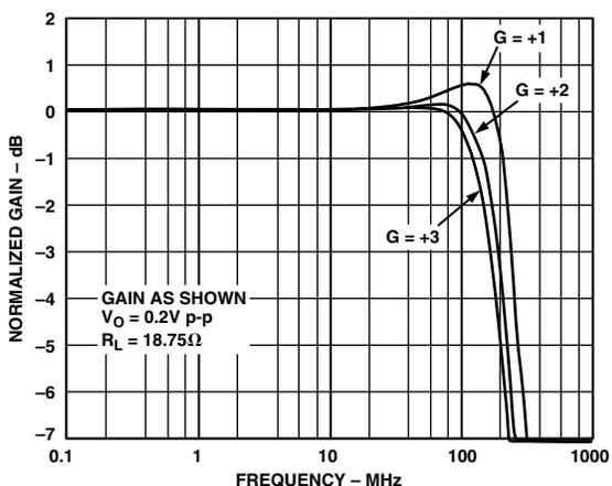
Figure 11. Small Signal Closed-Loop Frequency Response;  $R_L = 18.75 \Omega$
