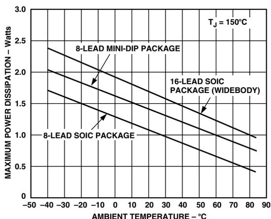
Figure 2. Plot of Maximum Power Dissipation vs. Temperature
