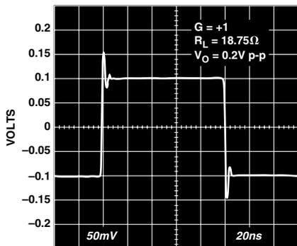
Figure 21. Small-Signal Pulse Response;  $G = +1$
