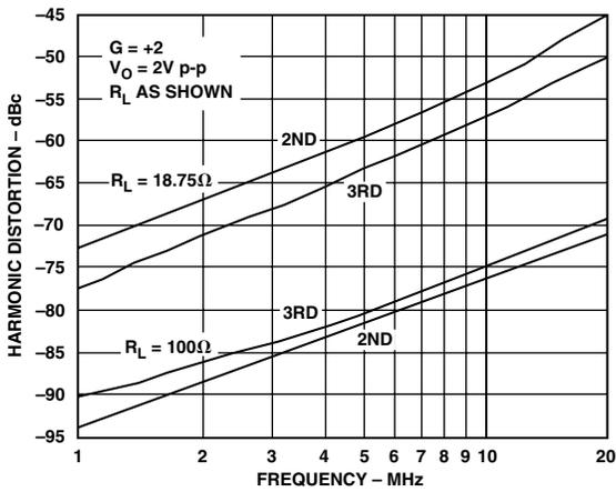
Figure 4. Harmonic Distortion vs. Frequency;  $G = +2$
