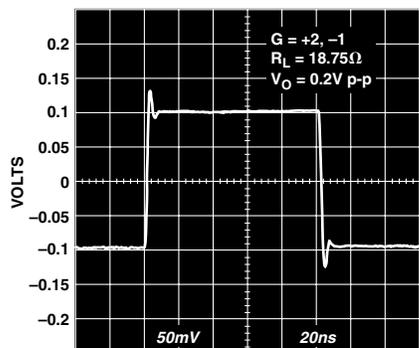
Figure 22. Small-Signal Pulse Response;  $G = +2, -1$
