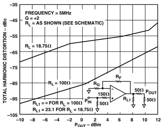
Figure 10. Total Harmonic Distortion vs.  $P_{OUT}$ ;  $G = +2$
