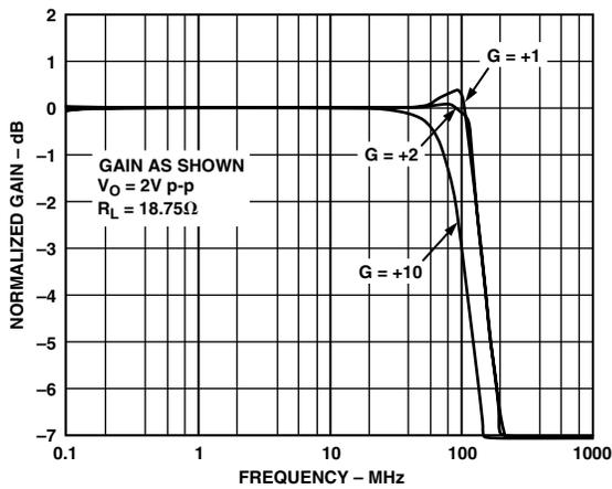
Figure 17. Large Signal Frequency Response;  $V_O = 2 V p-p$
