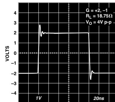
Figure 25. Large-Signal Pulse Response;  $G = +2, -1$
