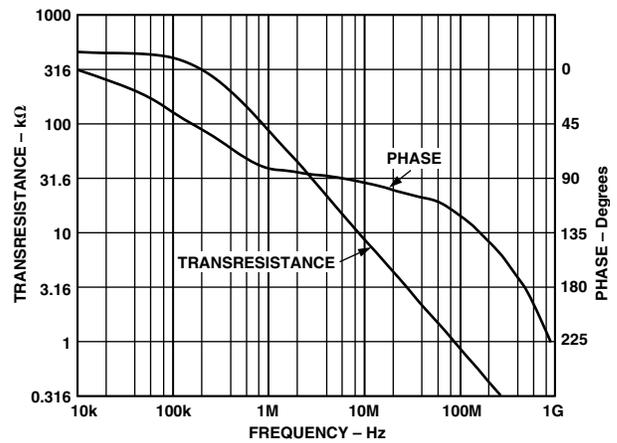
Figure 19. Transresistance and Phase vs. Frequency;  $R_L = 18.75 \Omega$
