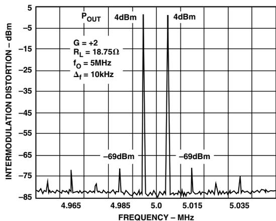
Figure 9. Intermodulation Distortion
