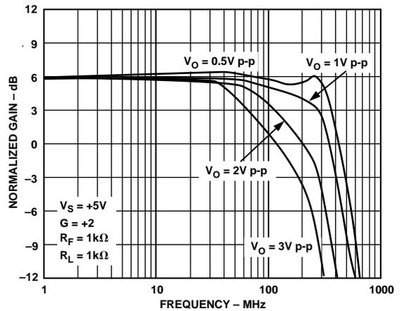
Figure 5. Bandwidth vs. Output Level—Single Supply,  $G = +2$
