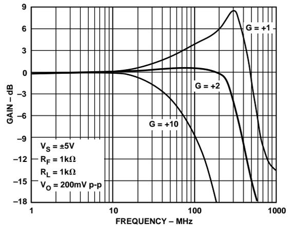
Figure 11. Bandwidth vs. Gain—Dual Supply,  $R_F = 1k\Omega$
