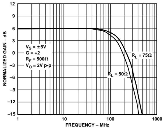
Figure 2. Frequency Response,  $G = +2$ ,  $V_O = 2\text{ V p-p}$
