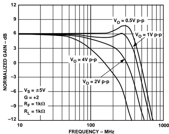
Figure 3. Bandwidth vs. Output Voltage Level—Dual Supply,  $G = +2$
