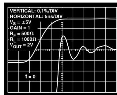
Figure 18. Settling Time
