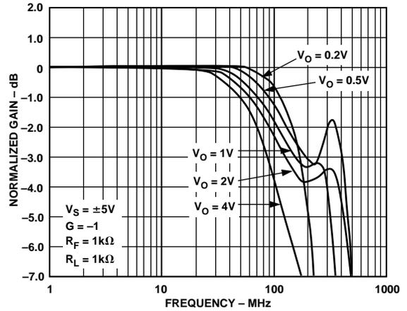
Figure 4. Bandwidth vs. Output Level—Gain of  $-1$ , Dual Supply
