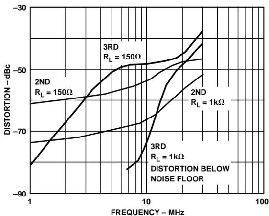
Figure 15. Distortion vs. Frequency;  $V_S = \pm 5 V$ ,  $G = +2$
