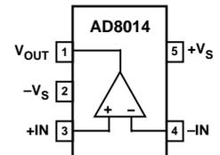
The AD8014 is a very high speed amplifier with 400 MHz, -3 dB bandwidth, 4000 V/ $\mu$ s slew rate, and 24 ns settling time. The AD8014 is a very stable and easy to use amplifier with fast overload recovery. The AD8014 has extremely low voltage and current noise, as well as low distortion, making it ideal for use in wide-band signal processing applications.
