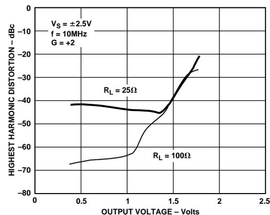
Figure 21. Distortion vs. Output Voltage,  $V_S = \pm 2.5\text{ V}$ ,  $G = +2$ ,  $f = 10\text{ MHz}$
