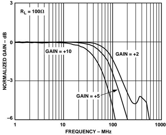
Figure 22. Frequency Response;  $V_S = \pm 6\text{ V}$
