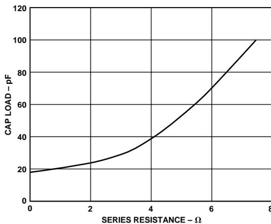
Figure 31.  $R_S$  and  $C_L$  vs. 30% Overshoot
