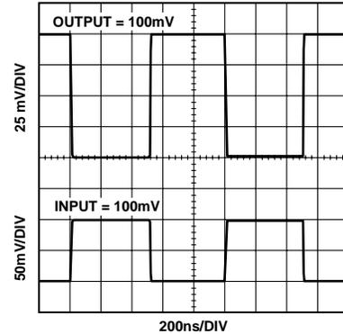
Figure 8. 100 mV Step Response;  $G = -1$ ,  $V_S = \pm 2.5$  V or  $\pm 6$  V,  $R_L = 100 \Omega$
