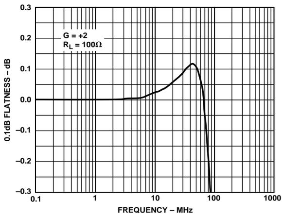
Figure 23. Gain Flatness;  $V_S = \pm 6\text{ V}$
