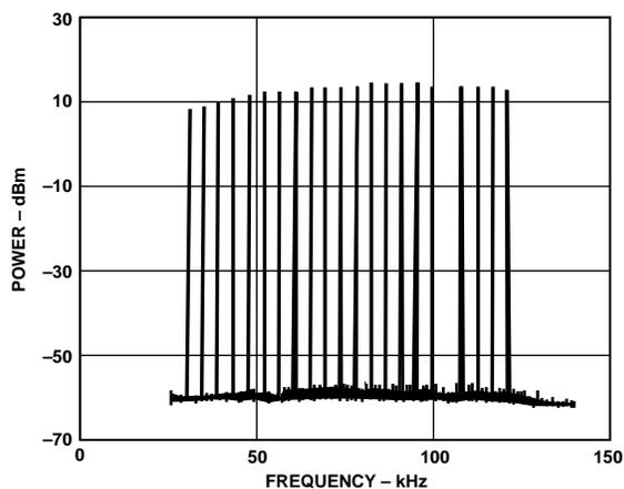
Figure 28. Multitone Power Ratio:  $V_S = \pm 6\text{ V}$ , 27 dBm Output Power into  $25\ \Omega$
