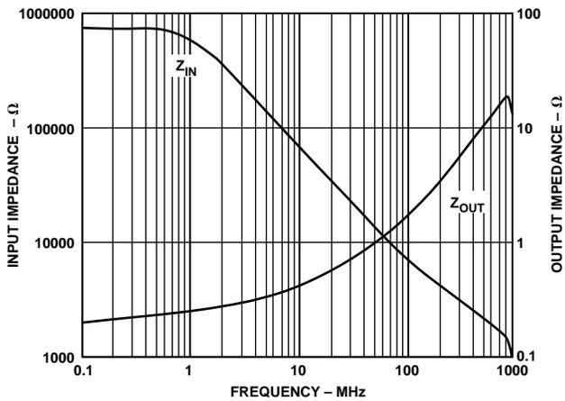
Figure 36. Input and Output Impedance vs. Frequency
