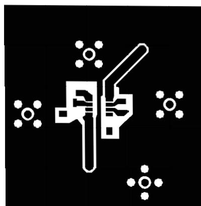
Figure 44. Universal SOIC Noninverter Bottom
