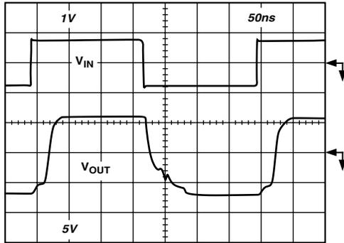
Figure 5. 15% Overload Recovery, Gain = +10
