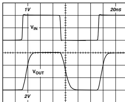
Figure 4. Pulse Response Driving a Large Load Capacitance,  $C_L = 300 \text{ pF}$ ,  $G = +3$ ,  $R_{FB} = 2.32 \text{ k}\Omega$ ,  $R_S = 10.5 \Omega$ ,  $R_L = 1 \text{ k}\Omega$ ,  $V_S = \pm 7.5 \text{ V}$
