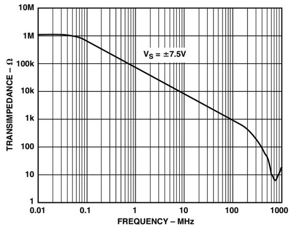
TPC 10. Open-Loop Transimpedance vs. Frequency,  $R_L = 150 \Omega$
