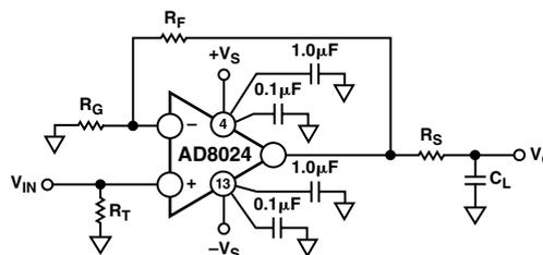
Figure 3. Circuit for Driving a Capacitive Load
