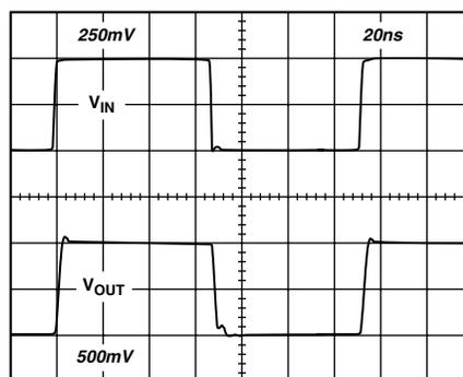
TPC 23. Small Signal Pulse Response, Gain = +2 ( $R_{FB} = 750 \Omega$ ,  $R_L = 150 \Omega$ ,  $V_S = \pm 7.5 \text{ V}$ )
