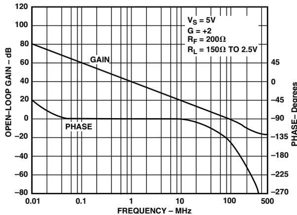
TPC 12. Open-Loop Gain and Phase vs. Frequency
