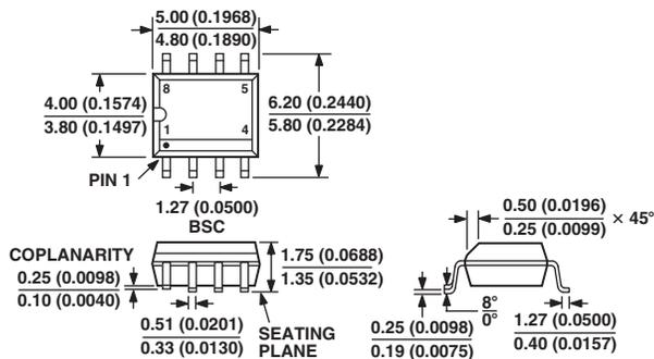
CONTROLLING DIMENSIONS ARE IN MILLIMETERS; INCH DIMENSIONS (IN PARENTHESES) ARE ROUNDED-OFF MILLIMETER EQUIVALENTS FOR REFERENCE ONLY AND ARE NOT APPROPRIATE FOR USE IN DESIGN
