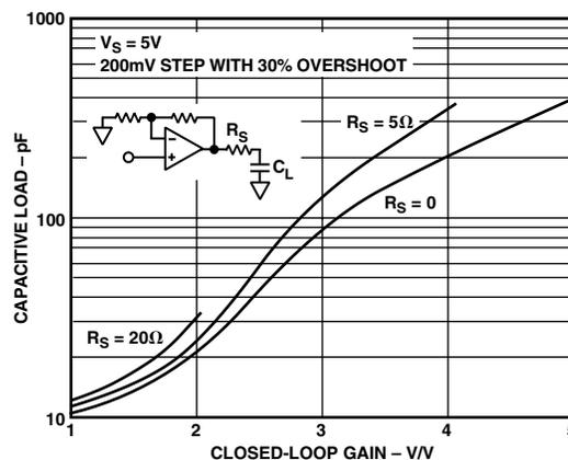
Figure 6. Capacitive Load Drive vs. Closed-Loop Gain
