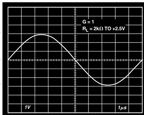
Figure 1. Output Swing: Gain =  $-1$ ,  $V_S = +5$  V
