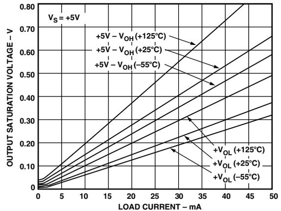
TPC 18. Output Saturation Voltage vs. Load Current
