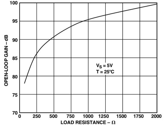
TPC 4. Open-Loop Gain vs.  $R_L$  to 2.5 V
