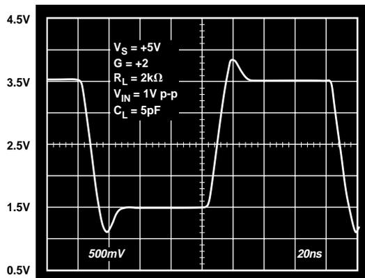
Figure 29. One Volt Step Response,  $V_S = +5V$ ,  $G = +2$
