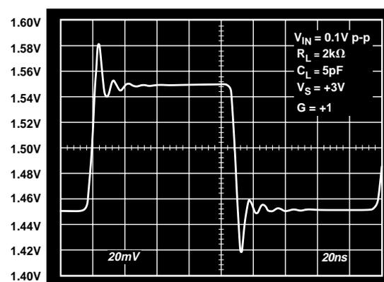
Figure 32. Step Response,  $G = +1$ ,  $V_{IN} = 100 \text{ mV}$
