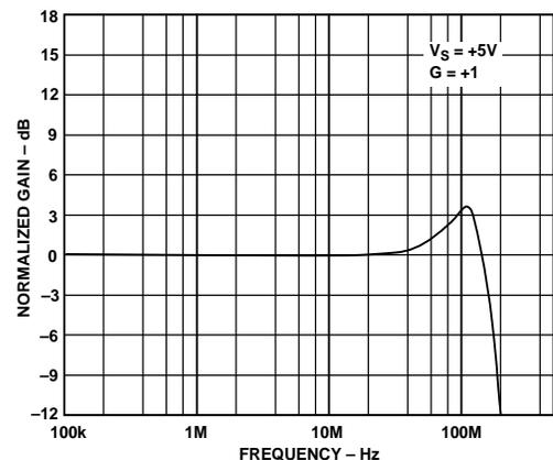
Figure 2. Frequency Response: Gain = +1,  $V_S = +5 \text{ V}$
