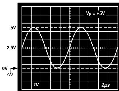
Figure 1. Output Swing: Gain = -1,  $R_L = 2 \text{ k}\Omega$
