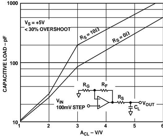
Figure 35. Capacitive Load Drive vs. Closed-Loop Gain
