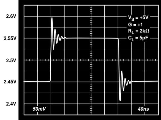
Figure 30. 100 mV Step Response,  $V_S = +5V$ ,  $G = +1$
