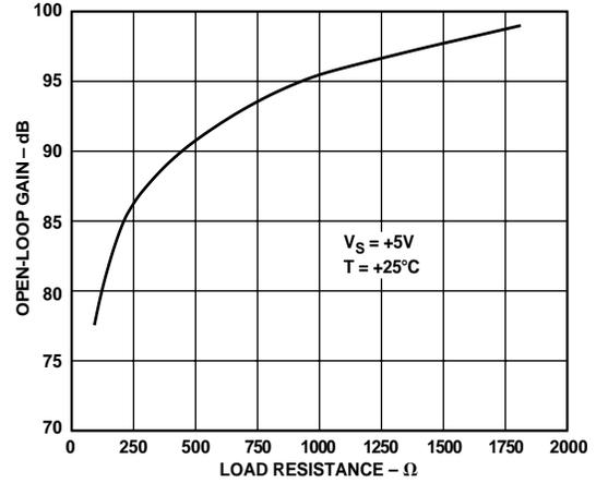
Figure 7. Open-Loop Gain vs.  $R_L$  to +2.5 V
