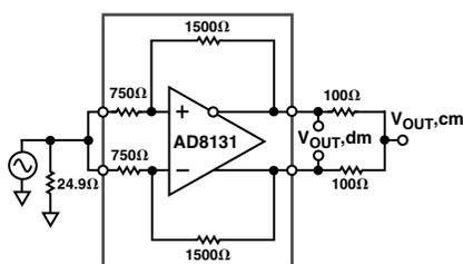
Figure 26. CMRR Test Circuit
