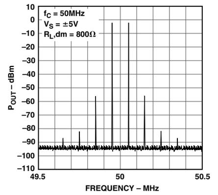
Figure 16. Intermodulation Distortion
