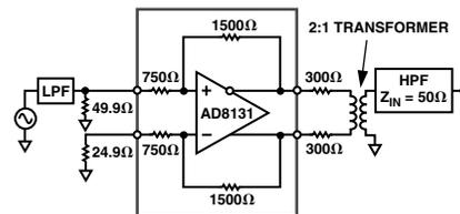
Figure 7. Harmonic Distortion Test Circuit ( $R_{L, dm} = 800\ \Omega$ )
