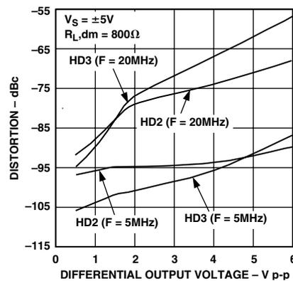
Figure 10. Harmonic Distortion vs. Differential Output Voltage
