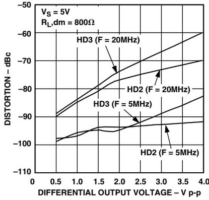
Figure 11. Harmonic Distortion vs. Differential Output Voltage
