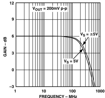
Figure 4. Small Signal Frequency Response
