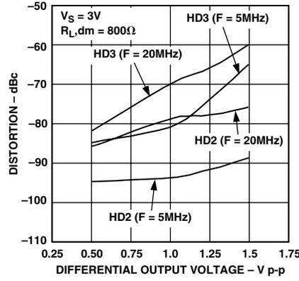
Figure 12. Harmonic Distortion vs. Differential Output Voltage
