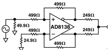
TPC 26. Test Circuit for Output Balance
