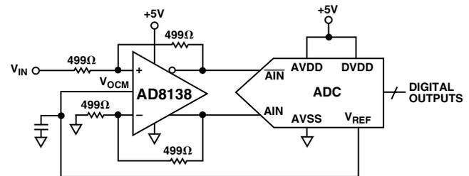
The AD8138 eliminates the need for a transformer with high performance ADCs, preserving the low frequency and dc information. The common-mode level of the differential output is adjustable by a voltage on the  $V_{OCM}$  pin, easily level-shifting the input signals for driving single-supply ADCs. Fast overload recovery preserves sampling accuracy.
