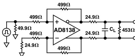
TPC 23. Test Circuit for Cap Load Drive
