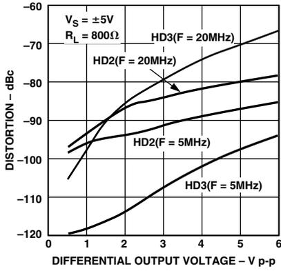
TPC 10. Harmonic Distortion vs. Differential Output Voltage
