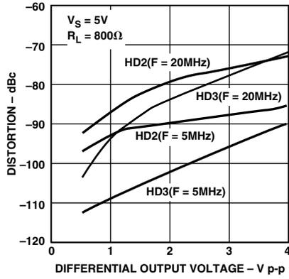
TPC 11. Harmonic Distortion vs. Differential Output Voltage
