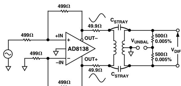
Figure 4. AD8138 Forms a Balanced Transformer Driver
