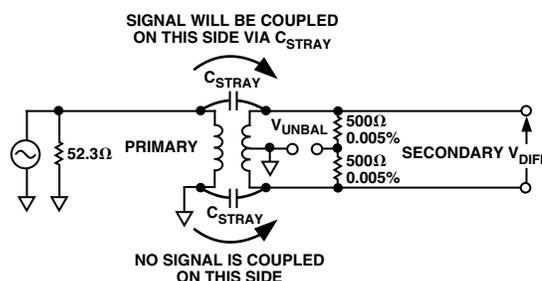
Figure 3. Transformer Single-Ended-to-Differential Converter Is Inherently Imbalanced
