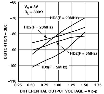
TPC 12. Harmonic Distortion vs. Differential Output Voltage
