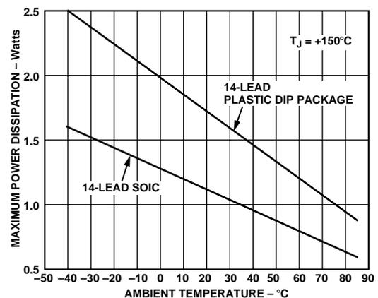
Figure 3. AD8182 Maximum Power Dissipation vs. Temperature
