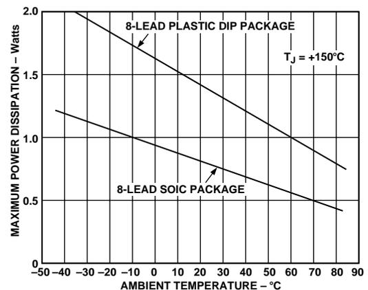
Figure 2. AD8180 Maximum Power Dissipation vs. Temperature
