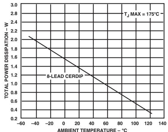
Figure 4. Maximum Power Dissipation vs. Temperature, CERDIP Package
