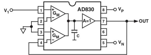
$V_{OUT} = V_1$
