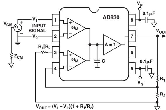
Figure 21. Gain of G Differential Amplifier,  $G > 1$
