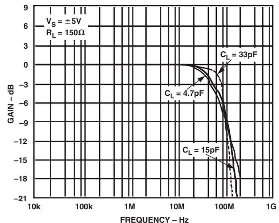
Figure 2. Closed-Loop Gain vs. Frequency, Gain = +1
