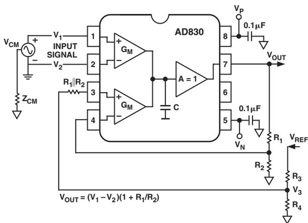
Figure 22. Offsetting the Output with Differential Gain > 1
