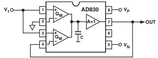
$V_{OUT} = 2V_1$
