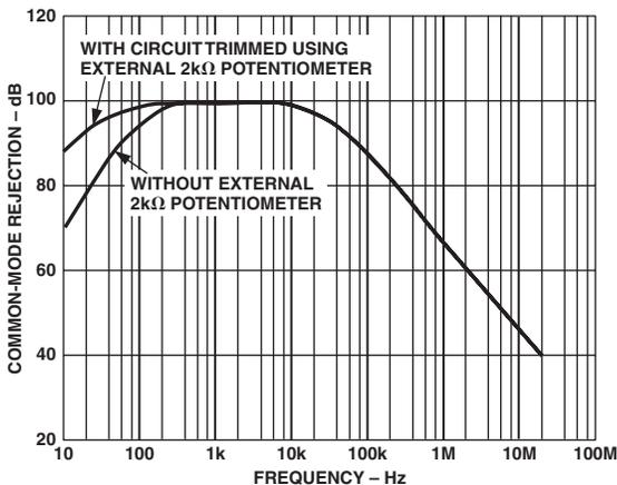
Figure 29. Common-Mode Rejection vs. Frequency for Line Receiver
