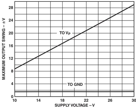
Figure 18. Output Swing Limit for Single Supply
