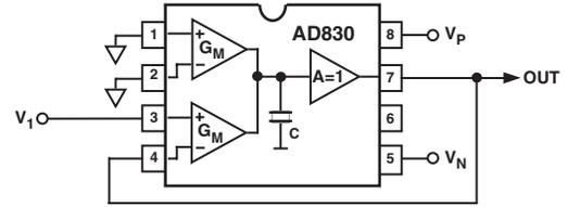
$V_{OUT} = V_1$
