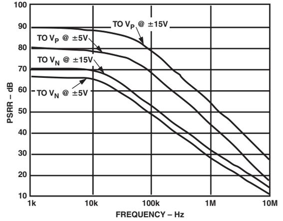
TPC 4. Power Supply Rejection Ratio vs. Frequency
