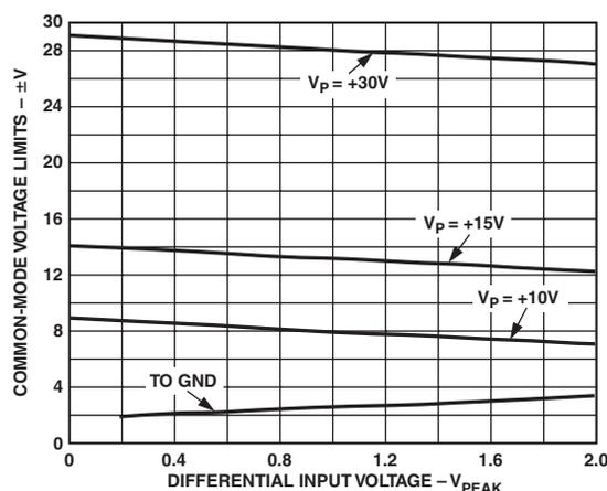
Figure 17. Input Common-Mode Range for Single Supply
