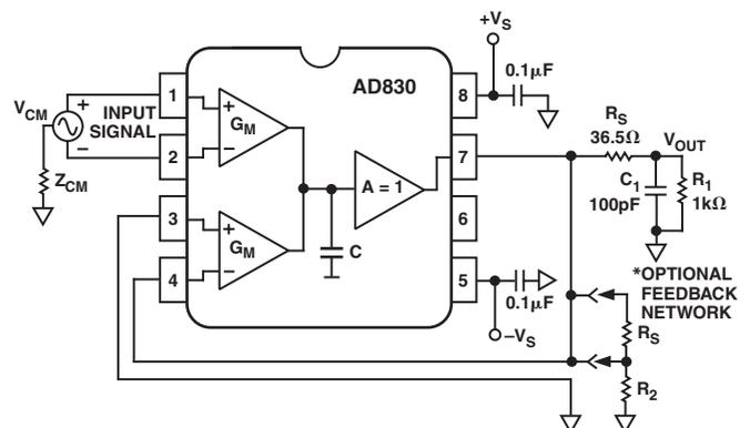
Figure 13. Circuit for Driving Large Capacitive Loads
