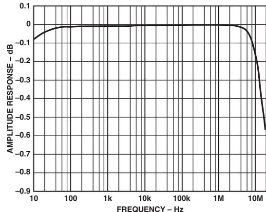
Figure 30. Amplitude Response vs. Frequency for Line Receiver
