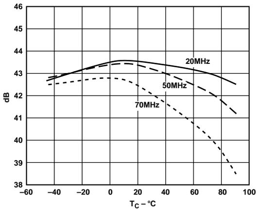
Figure 17. SINAD vs. Temperature:  $f_S = 200$  MSPS
