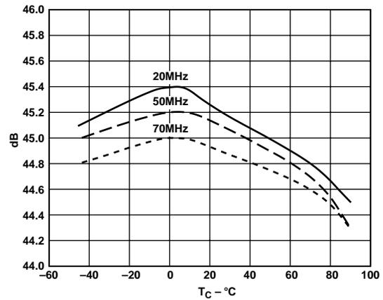
Figure 13. SNR vs. Temperature,  $f_S = 200$  MSPS
