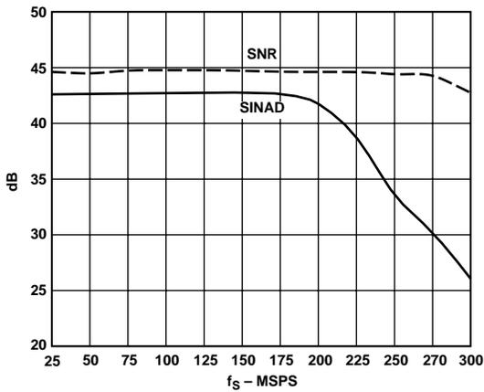
Figure 11. SNR vs.  $f_S$ :  $f_{IN} = 70.1$  MHz
