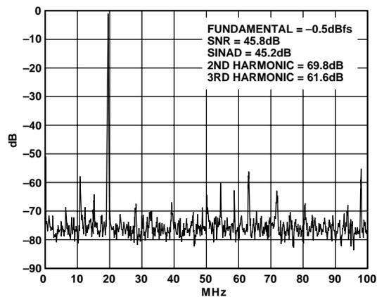
Figure 25. Spectrum:  $f_S = 200$  MSPS,  $f_{IN} = 19.7$  MHz
