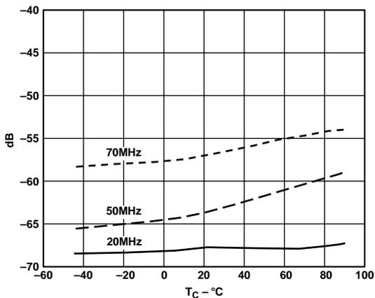
Figure 21. 2nd Harmonic vs. Temperature:  $f_S = 200$  MSPS
