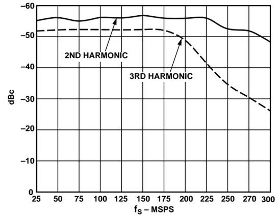
Figure 19. Harmonic Distortion vs.  $f_S$ :  $f_{IN} = 70.1$  MHz
