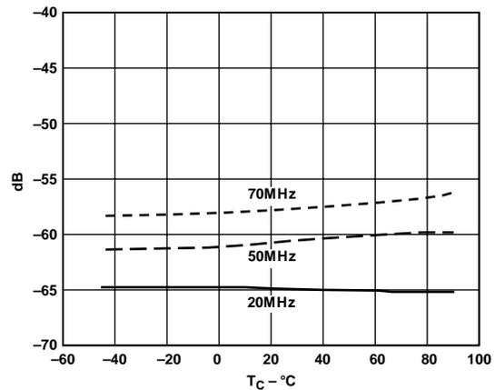
Figure 20. 2nd Harmonic vs. Temperature:  $f_S = 135$  MSPS
