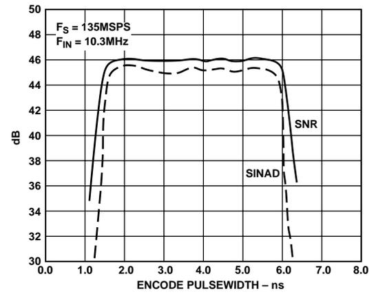
Figure 14. SNR vs. Clock Pulsewidth, ( $t_{PWH}$ ):  $f_S = 135$  MSPS
