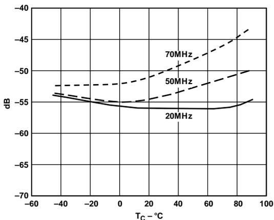
Figure 23. 3rd Harmonic vs. Temperature:  $f_S = 200$  MSPS
