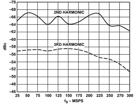
Figure 18. Harmonic Distortion vs.  $f_S$ :  $f_{IN} = 19.7$  MHz
