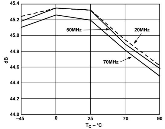
Figure 12. SNR vs. Temperature,  $f_S = 135$  MSPS
