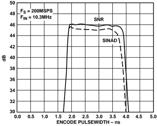
Figure 15. SNR vs. Clock Pulsewidth, ( $t_{PWH}$ ):  $f_S = 200$  MSPS
