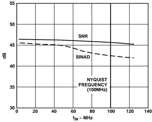
Figure 9. SNR vs.  $f_{IN}$ :  $f_S = 200$  MSPS
