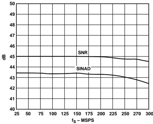
Figure 10. SNR vs.  $f_S$ :  $f_{IN} = 19.7$  MHz
