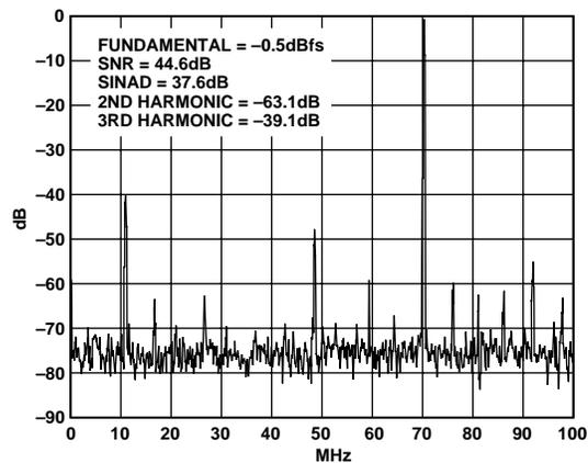
Figure 26. Spectrum:  $f_S = 200$  MSPS,  $f_{IN} = 70.1$  MHz
