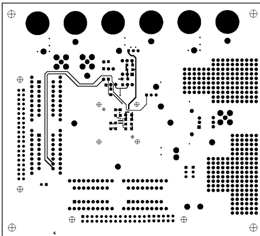
Figure 41. Evaluation Board, Bottom Layer
