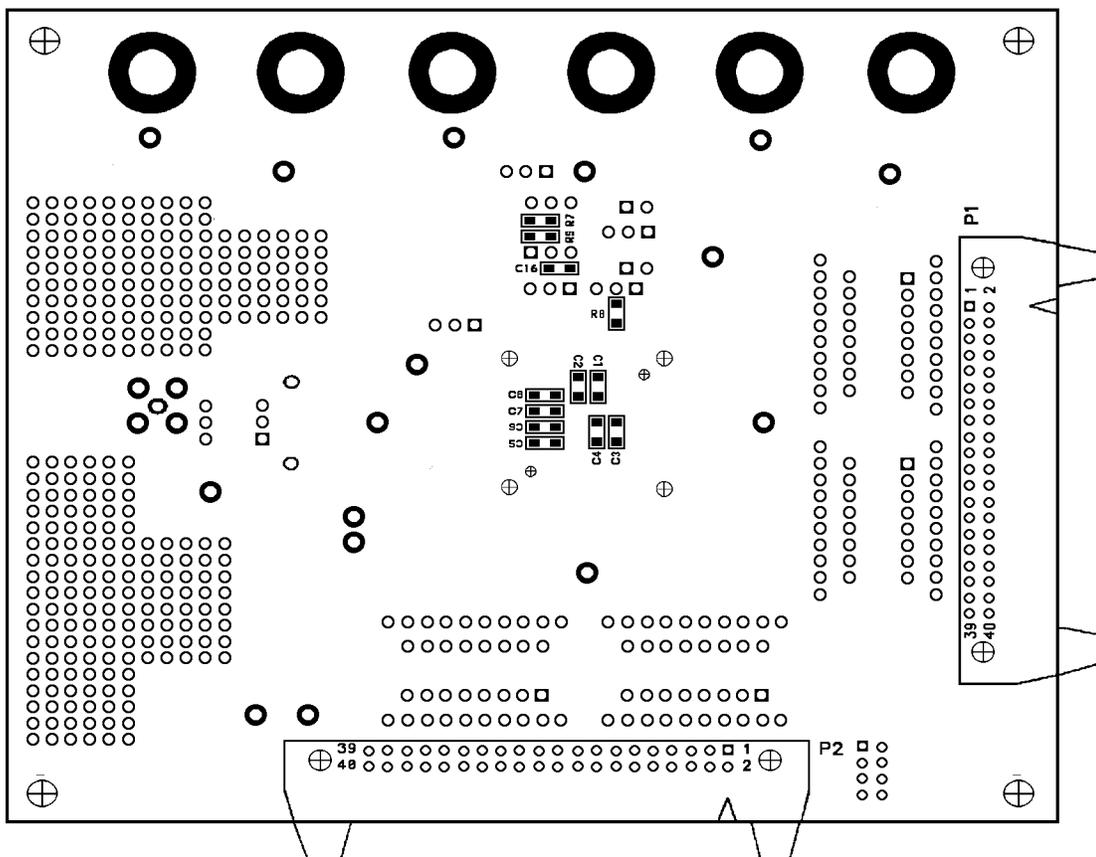
Figure 37. Evaluation Board, Assembly – Bottom
