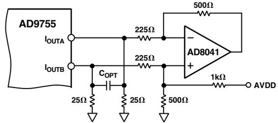
Figure 22. Single Supply DC Differential Coupled Circuit
