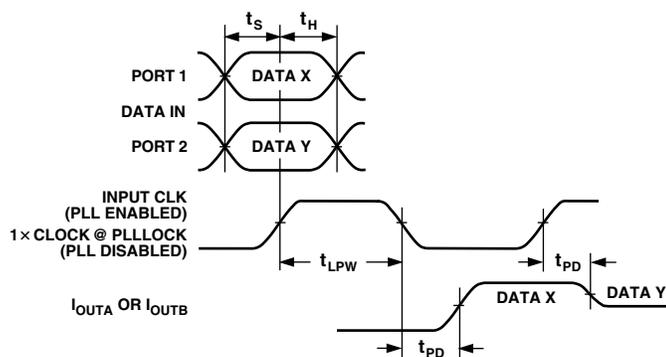
Figure 1. I/O Timing
