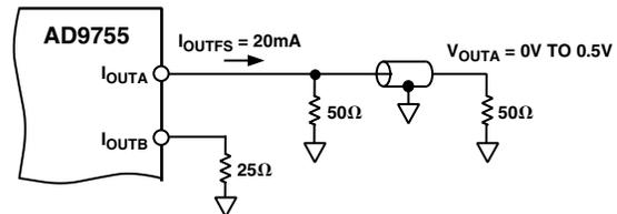
Figure 23. 0 V to 0.5 V Unbuffered Voltage Output
