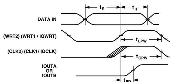
Figure 1. Timing Diagram for Dual and Interleaved Modes
