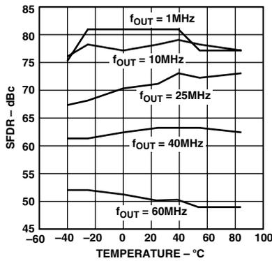
Figure 15. SFDR vs. Temperature @  $125 \text{ MSPS}$ ,  $0 \text{ dBFS}$
