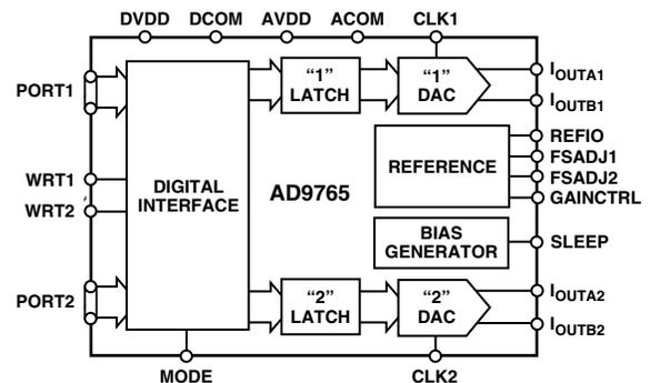
and provide a nominal full-scale current of 20 mA. The full-scale currents between each DAC are matched to within 0.1%.
