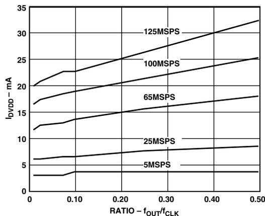
Figure 31.  $I_{DVDD}$  vs. Ratio @  $DVDD = 5$  V
