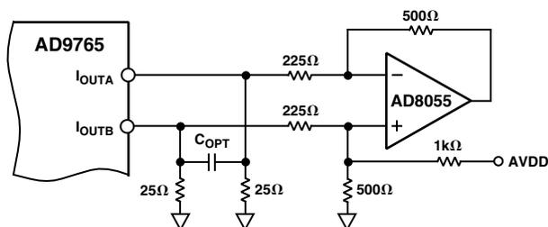
Figure 35. Single Supply DC Differential Coupled Circuit
