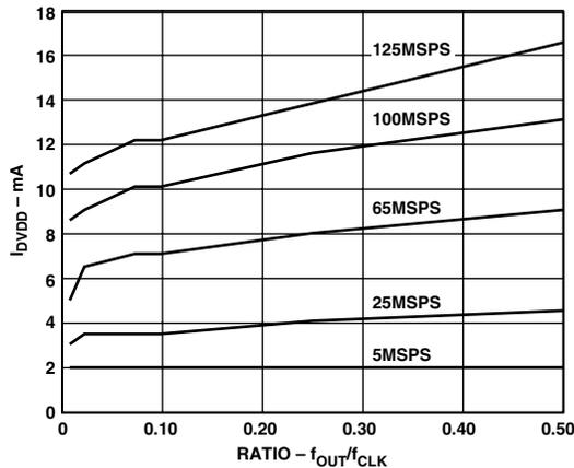
Figure 32.  $I_{DVDD}$  vs. Ratio @  $DVDD = 3V$
