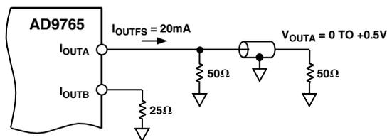
Figure 36. 0 V to 0.5 V Unbuffered Voltage Output
