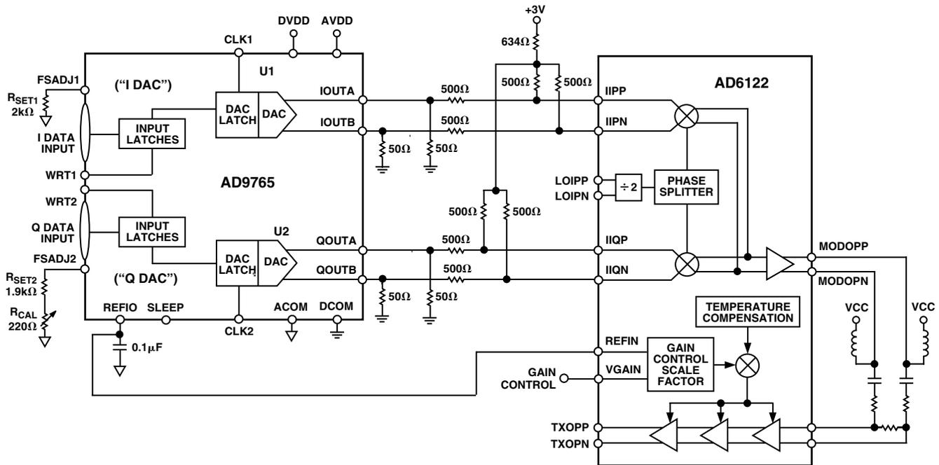
Figure 44. CDMA Transmit Application Using AD9765 and AD6122
