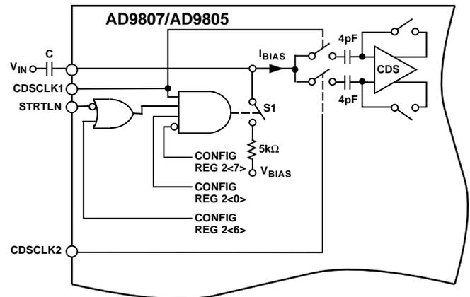
Figure 17. Equivalent Analog Inputs (VINR, VING, and VINB)
