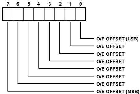
Figure 10. Odd and Even Offset Registers Format
