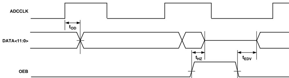
Figure 11. Digital Output Timing
