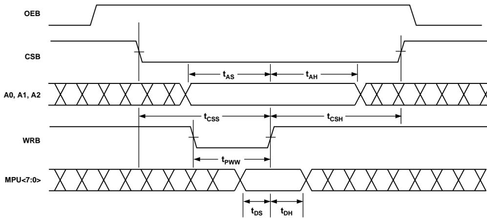
Figure 2. Write Timing
