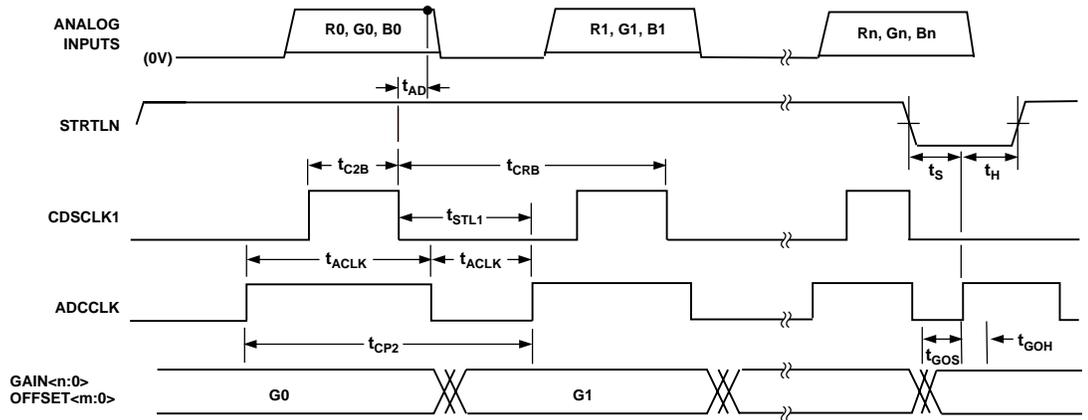
Figure 1f. 1-Channel SHA-Mode Clock Timing (Red Channel)
