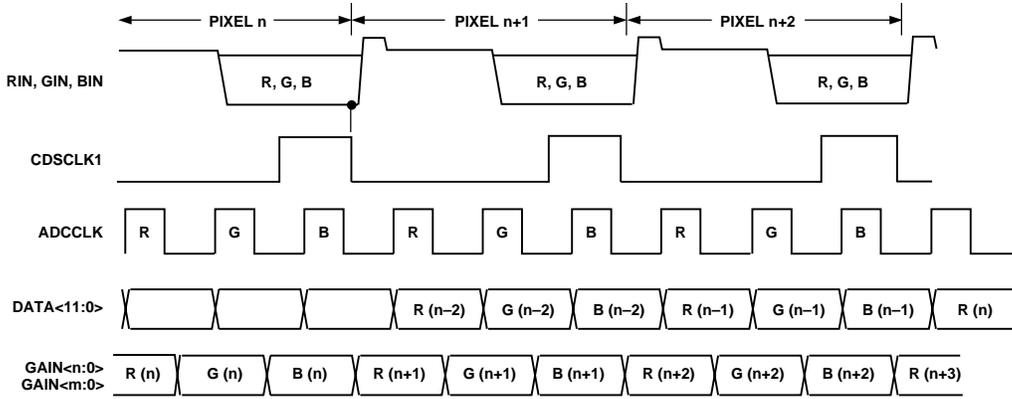
Figure 13. DOUT Latency, 3-Channel SHA Mode
