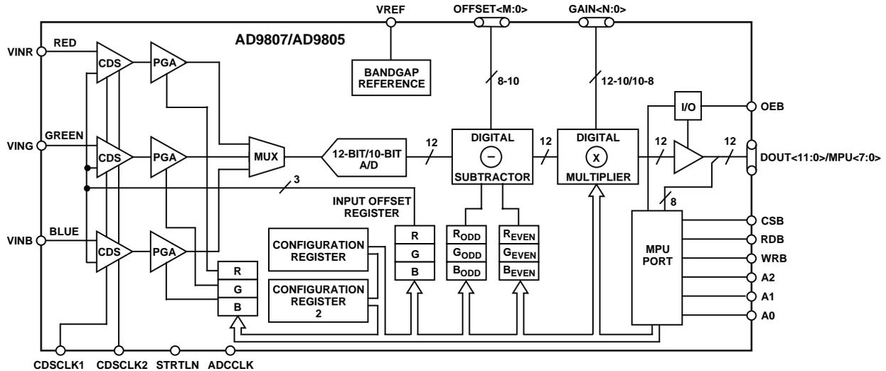
Figure 4. Block Diagram
