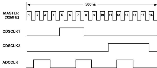
Figure 18. Timing Scheme Using 16  $\times$  Master Clock
