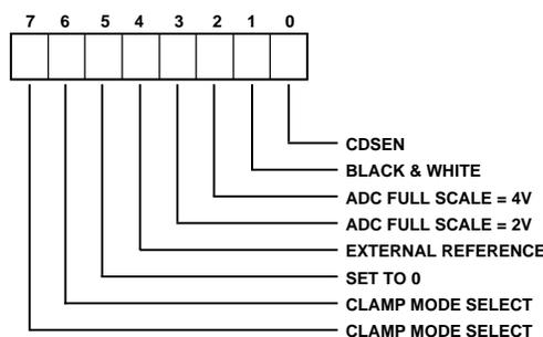
Figure 7. AD9807/AD9805 Configuration Register 2 Format
