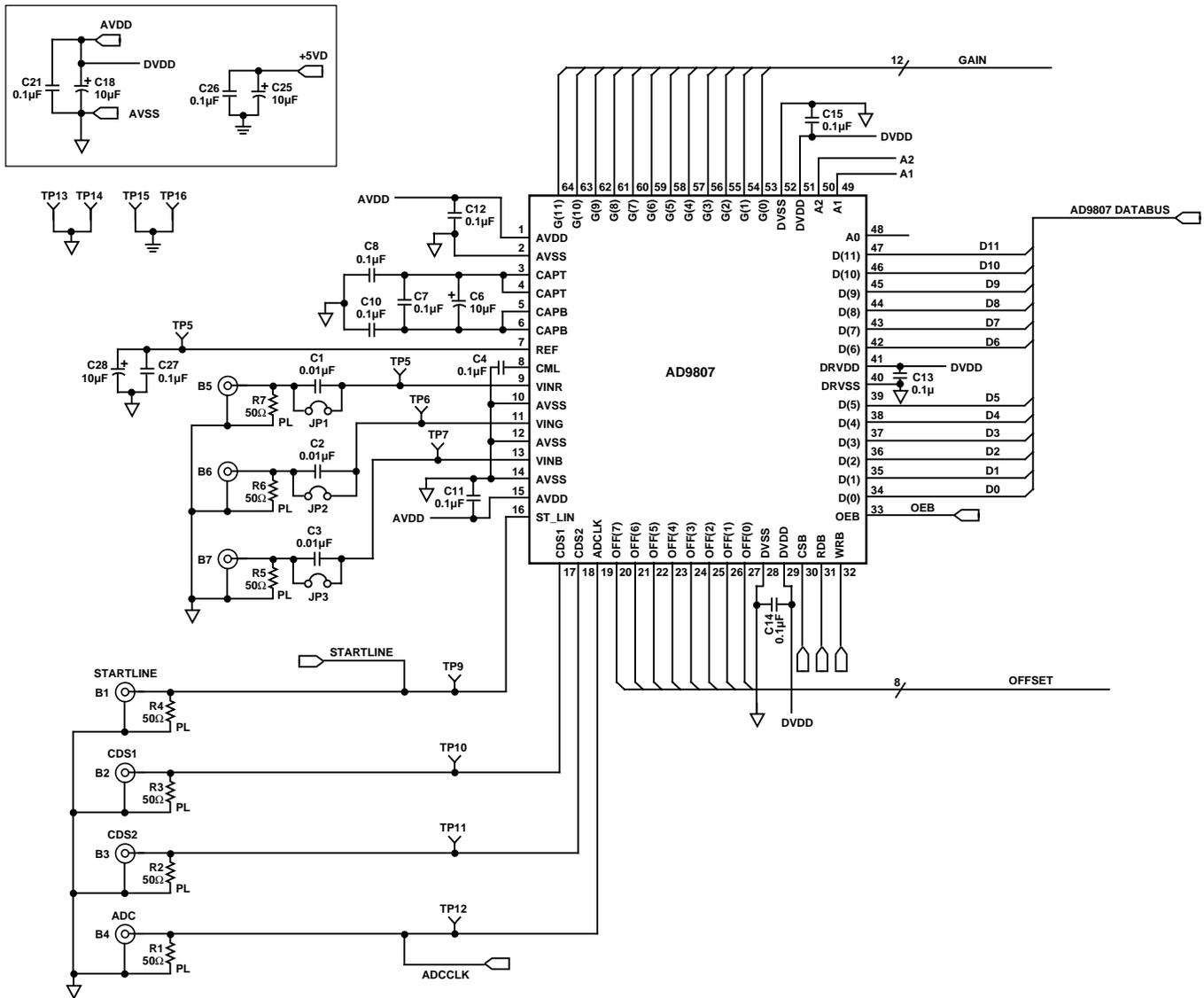
Figure 26. AD9807 Evaluation Board (Digital Circuitry Omitted)
