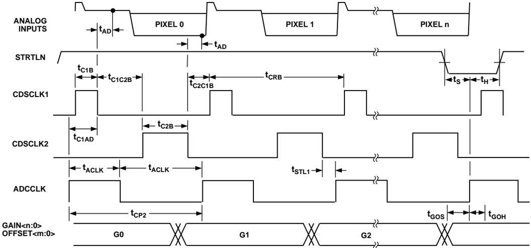
Figure 1d. 1-Channel CDS-Mode Clock Timing (Red Channel)
