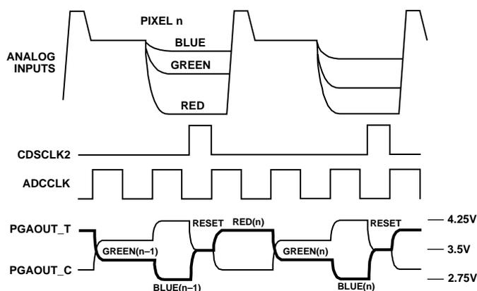
Figure 18. PGA Output Voltages (ADC Input Range = 3 V)
