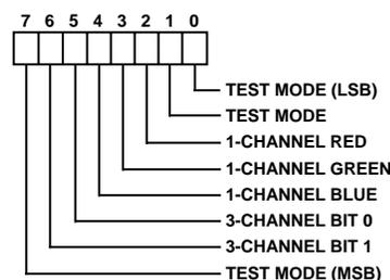
Figure 8. MUX Register
