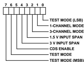
Figure 7. Configuration Register
