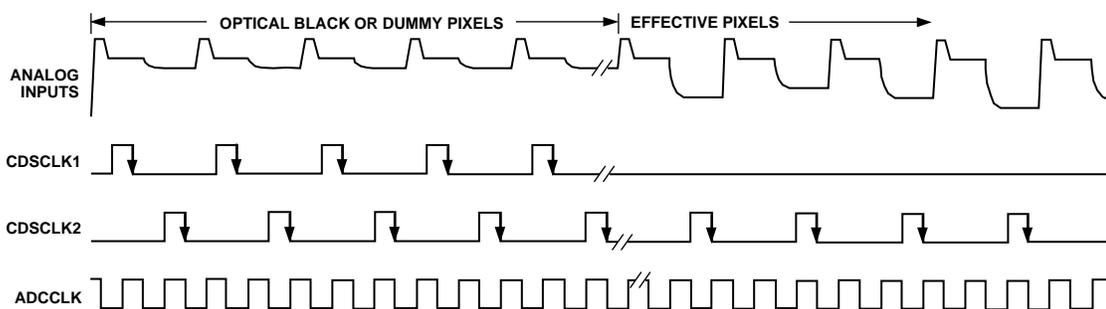
Figure 5. Line Clamp Timing for 3-Channel CDS Mode
