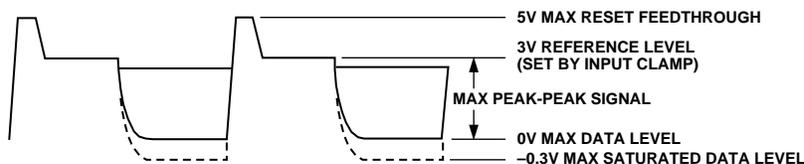
Figure 14. CCD Input Signal Clamped to 3 V
