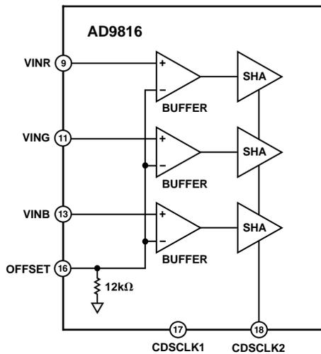
Figure 15. SHA Mode Input Circuit
