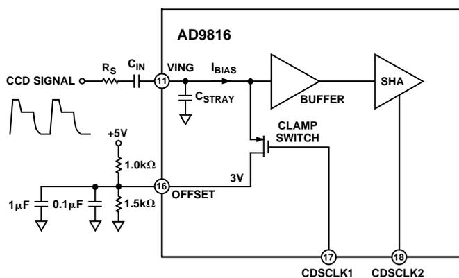
Figure 13. CDS Mode Input Circuit (All Channels Identical)
