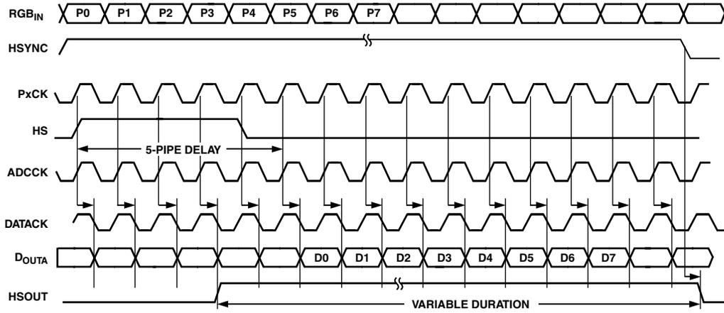
Figure 8. 4:4:4 Mode (For RGB and YUV)
