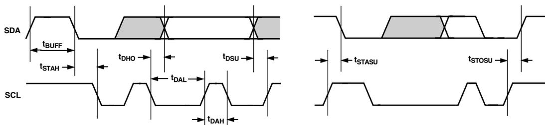
*Figure 10. Serial Port Read/Write Timing*
