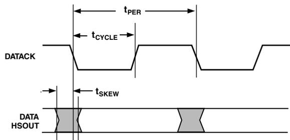
Figure 7. Output Timing
