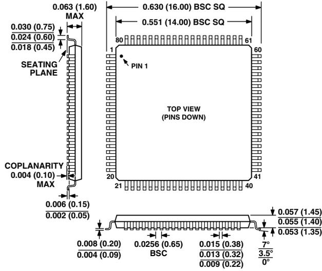
CONTROLLING DIMENSIONS IN MILLIMETERS.
