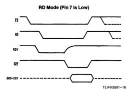
When in RD mode, the comparator phases are internally triggered. At the falling edge of RD, the MS flash converter goes from zero to compare mode and the LS ADC's comparators enter their zero cycle. After 800 ns, data from the MS flash is latched and the LS flash ADC enters compare mode. Following another 800 ns, the lower 4 bits are recovered.
