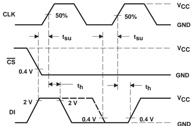
Figure 1. ADC0832 Data Input Timing
