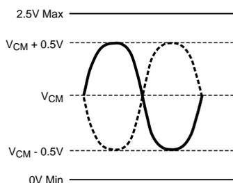
**Figure 38. Input Voltage Waveforms for a 2V<sub>p-p</sub> differential Input**
