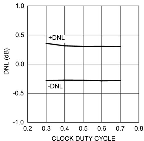
Figure 6. DNL vs. Clock Duty Cycle (DC input)
