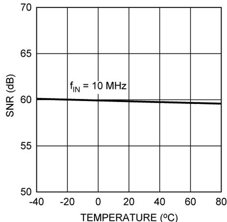
Figure 16. SNR vs. Temperature
