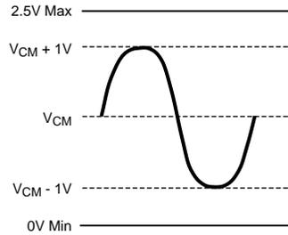
**Figure 39. Input Voltage Waveform for a 2V<sub>p-p</sub> Single Ended Input**
