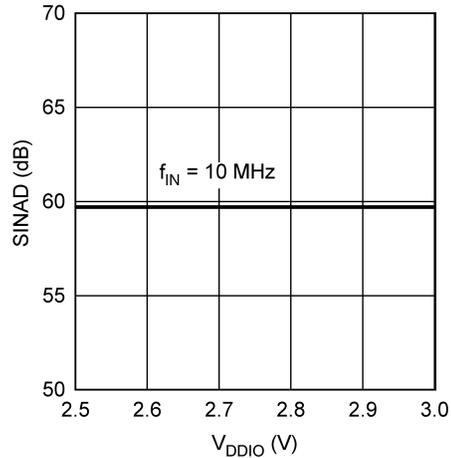
Figure 23. SINAD vs. V<sub>DDIO</sub>
