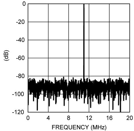
Figure 35. Spectral Response @ 11 MHz Input
