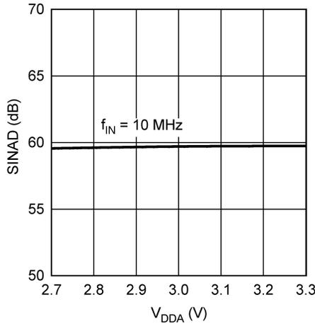
Figure 22. SINAD vs. V<sub>DDA</sub>
