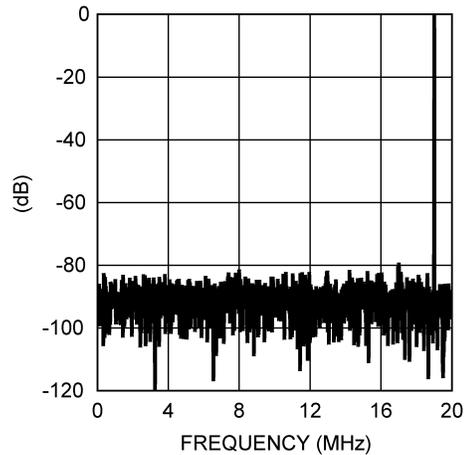
Figure 37. Spectral Response @ 19 MHz Input
