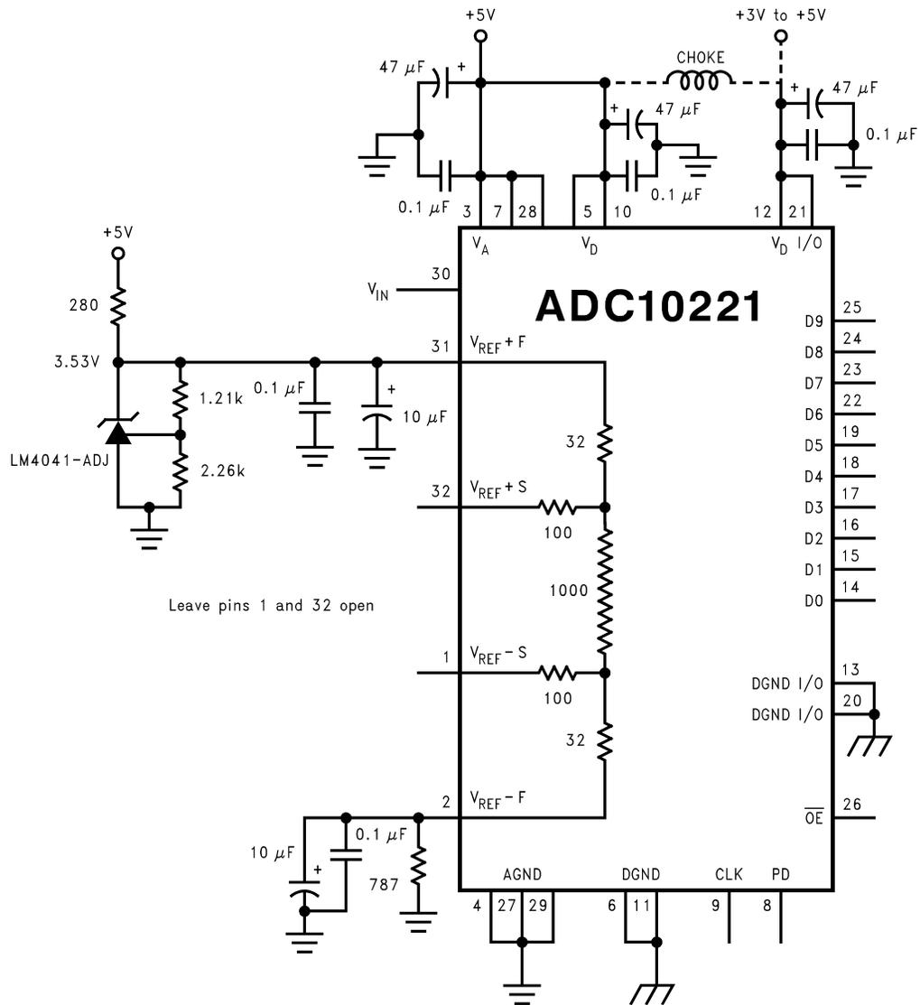
Figure 18. Simple, low component count reference biasing
