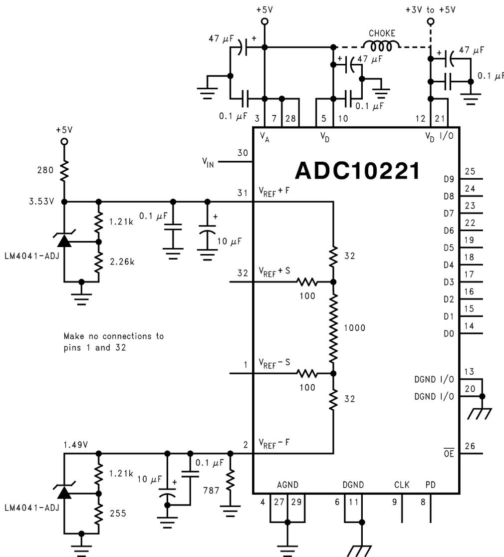
Figure 19. Better low component count reference biasing
