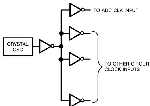
**Figure 22. Isolating the ADC clock from digital circuitry**
