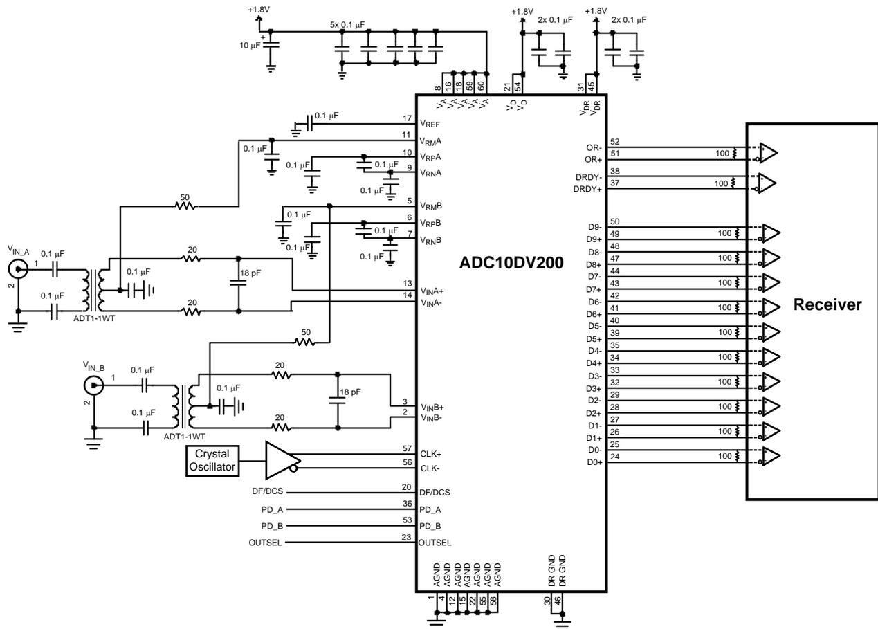
Figure 27. Application Circuit
