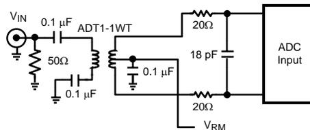
**Figure 25. Low Input Frequency Transformer Drive Circuit**
