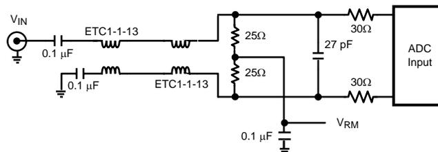
**Figure 26. High Input Frequency Transformer Drive Circuit**
