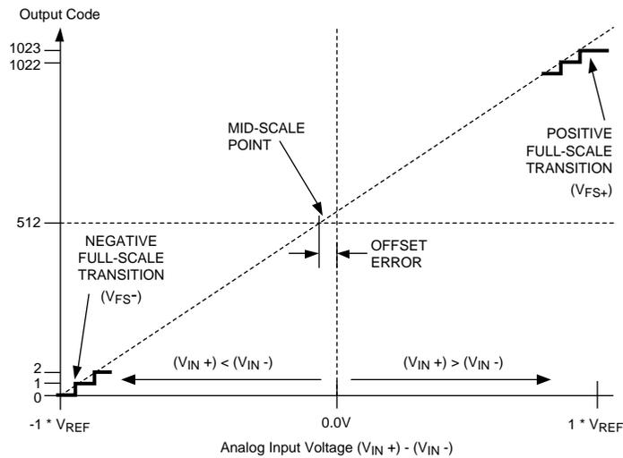
Figure 3. Transfer Characteristic
