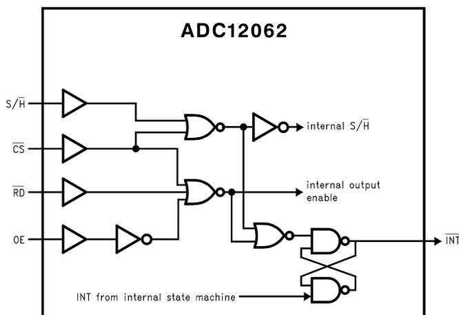
Figure 8. ADC Control Logic
