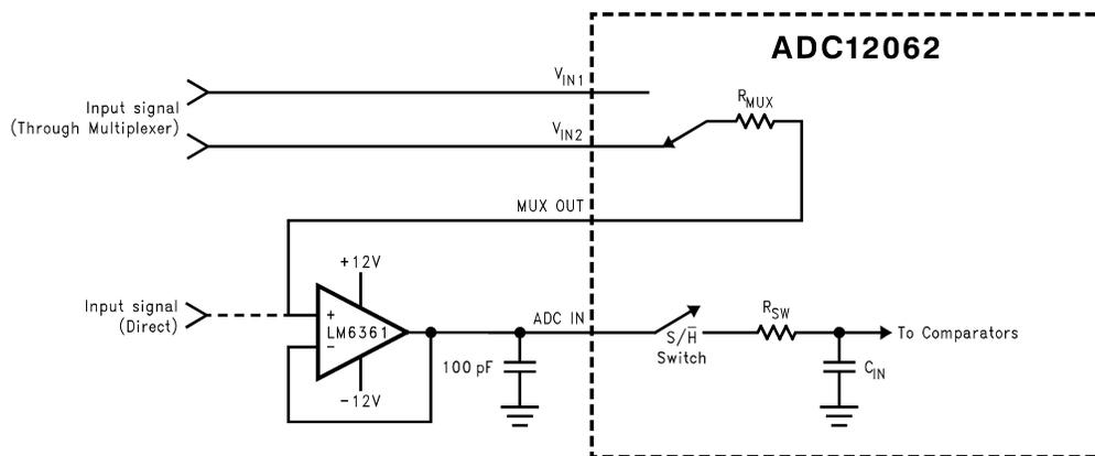
Figure 10. Buffering the Input with an LM6361 High Speed Op Amp
