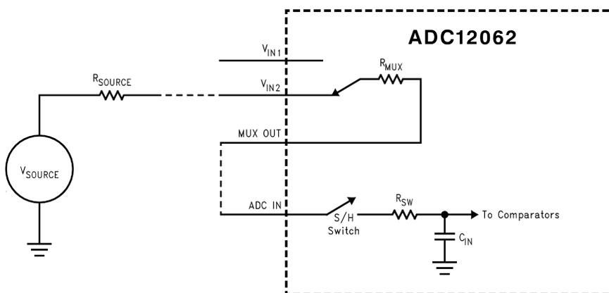
Figure 9. Simplified ADC12062 Input Stage
