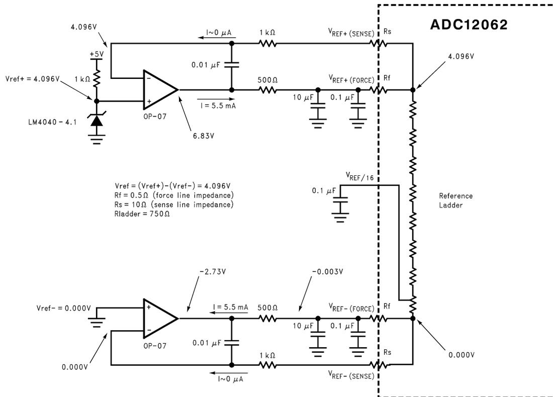
Figure 12. Reference Ladder Force and Sense Inputs
