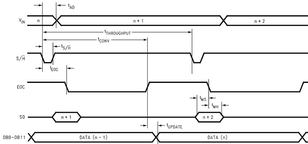
Figure 2. High Speed Interface Timing (MODE = 1, OE = 1, CS = 0, RD = 0)
