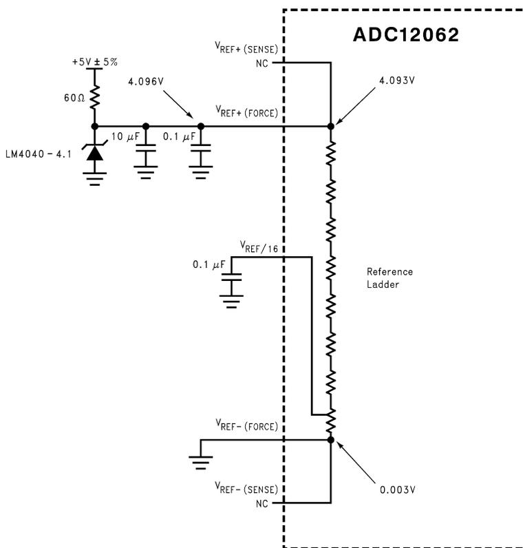
Figure 13. Using the  $V_{REF}$  Force Pins Only
