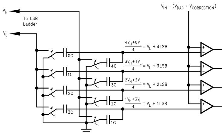
Figure 7. The Capacitive Voltage Divider
