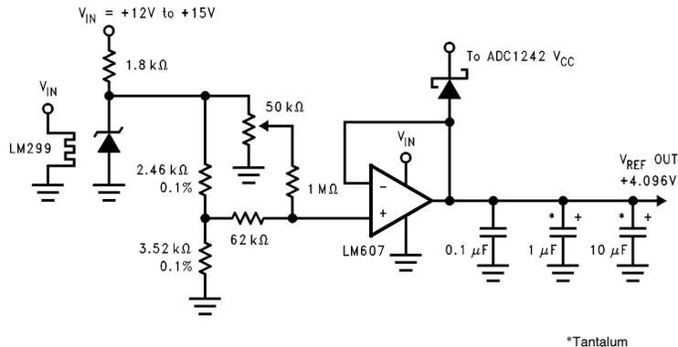
FIGURE 4. Low Drift Extremely Stable Reference Circuit
