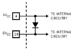
To guarantee accuracy, it is required that the  $AV_{CC}$  and  $DV_{CC}$  be connected together to a power supply with separate bypass filters at each  $V_{CC}$  pin.
