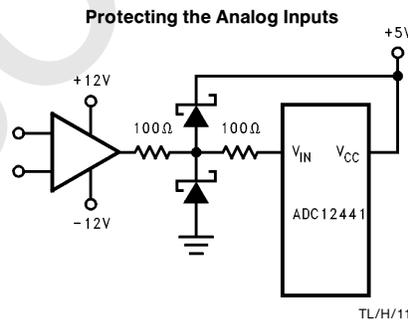
**Note:** External protection diodes should be able to withstand the op amp current limit.
