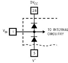
This means that if  $AV_{CC}$  and  $DV_{CC}$  are minimum ( $4.75 V_{DC}$ ) and  $V^-$  is maximum ( $-4.75 V_{DC}$ ), full-scale must be  $\leq 4.8 V_{DC}$ .
