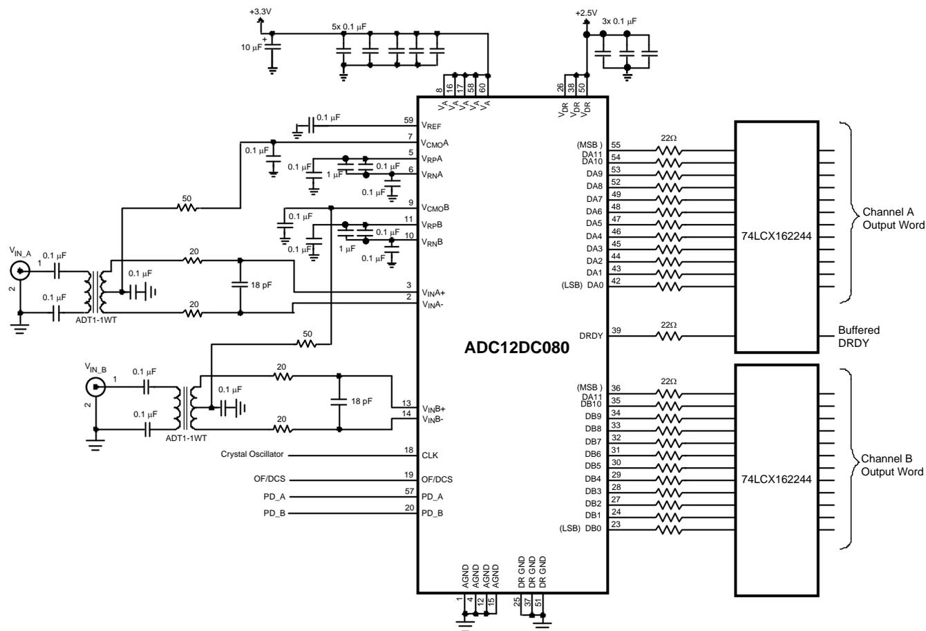
Figure 21. Application Circuit
