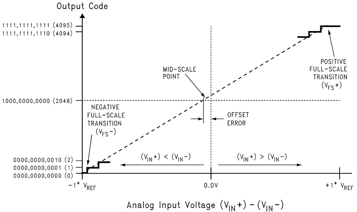
**Figure 2. Transfer Characteristic**
