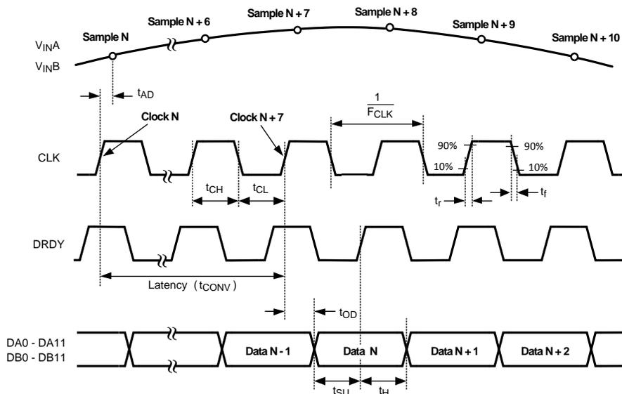
Figure 1. Output Timing
