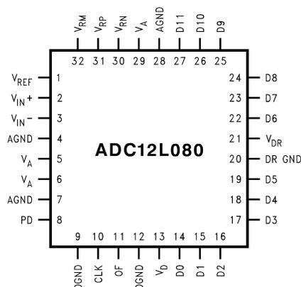
**Figure 1. 32-Lead LQFP Package**
