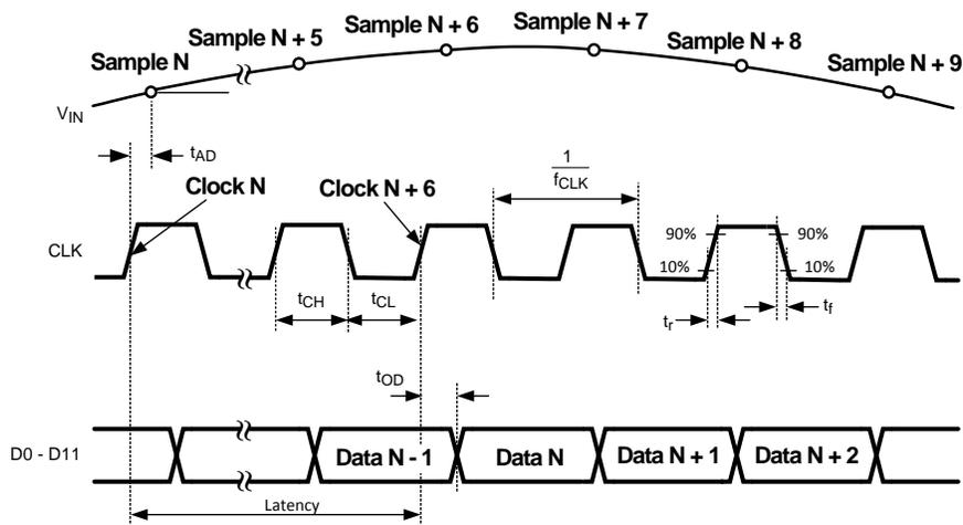
Figure 2. Output Timing
