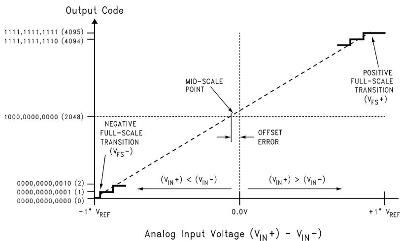
Figure 3. Transfer Characteristic
